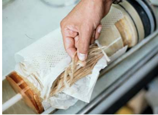
Figure 1 Fabric in hollow fine fibre permeator of Du Pont Permasep (Jan C. Schippers)
