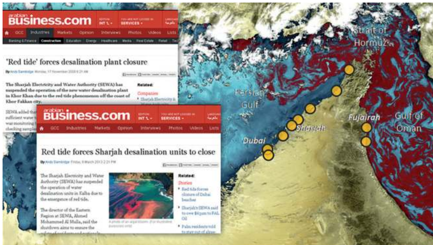
Figure 1 A “red tide” algal bloom off the coast of Oman, UAE and Iran as illustrated in this enhanced image based from the satellite image obtained by the European Space Agency MERIS FR satellite on 22 November 2008 (Planetek Hellas/ESA). Yellow points indicate locations of large RO plants in the area. Inset screenshots of online news regarding RO desalination plant shutdowns in the area in 2008 and 2013 ( www.arabianbusiness.com ).
