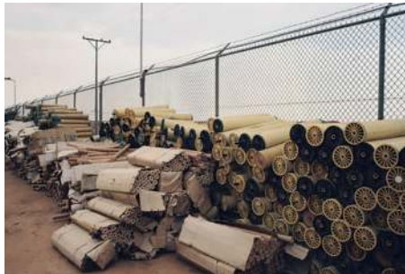
Figure 1 Old reverse osmosis elements and cartridge filters piling up before final disposal. (Jan C. Schippers)
