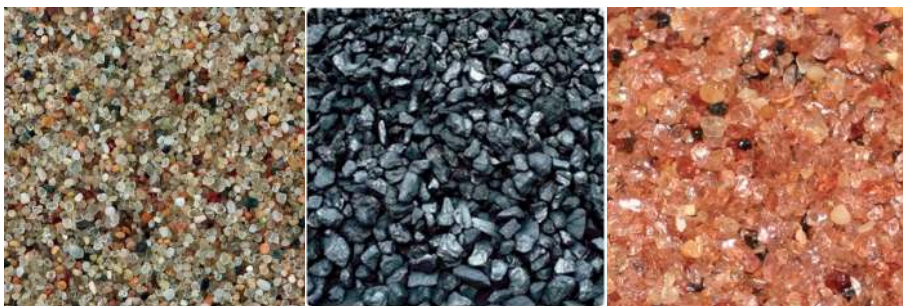
Figure 7 Photographs of sand media, anthracite media, and garnet media (Sharma and Schippers , 2019)
