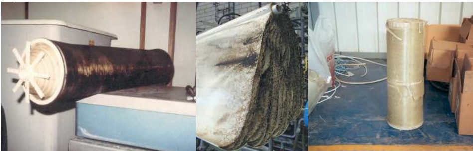
Figure 2 Telescoping (left), channelling (middle) and squeezing (right) of RO elements. (Jan C. Schippers)
