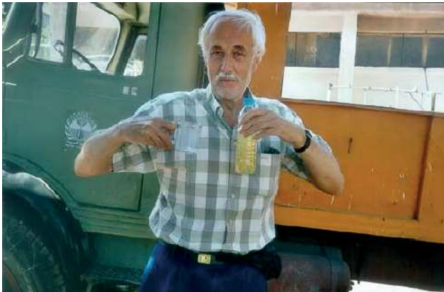
Figure 3 Groundwater samples immediately after sampling (left) and a couple of minutes after aeration (right). Location: Baq'a, Amman, Jordan (Jan C. Schippers).
