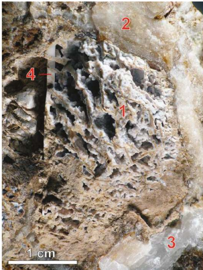
Figure 7. Beryllite (1) pseudomorph after chkalovite, in albite (2), from an aegirine-feldspar lens in sodalite-nepheline syenite, Mt Karnasurt, Lovozero. (3)—Natrolite, (4)—microcline.
