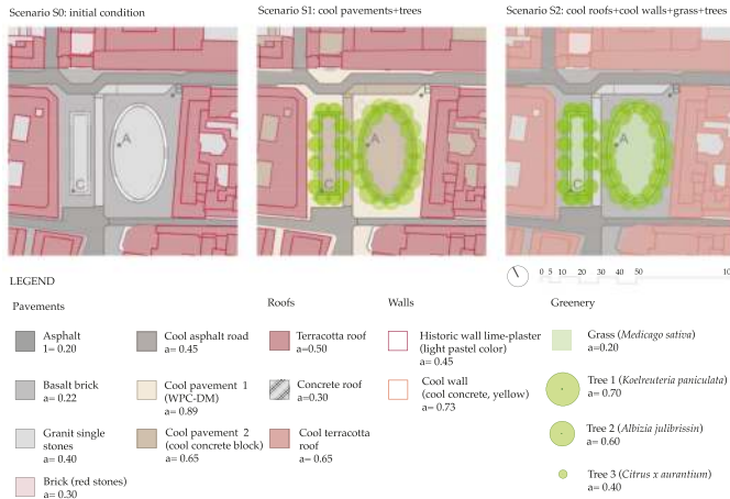
Figure 2. Initial condition scenario S0 (a), first renovation scenario S1 (b), second renovation scenario S2 (c). Point A, B and C represent the selected location for the comparisons among the scenarios.
