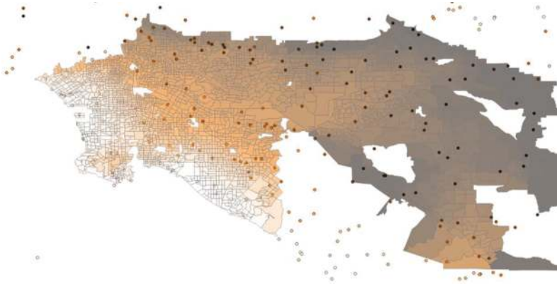
Figure 3. Los Angeles region model UHII (background) and mesonet observation (small circles) at 320 stations in this domain for June 2013. Both model UHII and observations are in DH/day ( ^\circ\text{C}\cdot\text{h}/\text{day} ). Lightest color is 6 \text{ }^\circ\text{C}\cdot\text{hr}/\text{day} ; darkest color is 190 \text{ }^\circ\text{C}\cdot\text{hr}/\text{day} . Compare the color changes of the small circles (mesonet observations) with those of the background UHII which shows a good agreement between the two.
