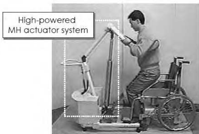
Fig. 19. Photograph of a prototype mobile floor hoist for transfer assistance.
