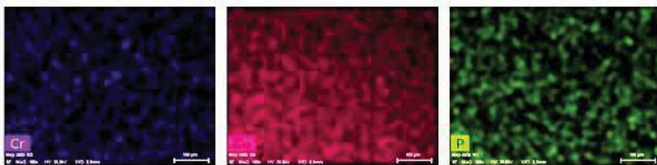
Figure 2. Distribution of Cu, Cr, and P in the CuCr0.6 alloy after casting.
