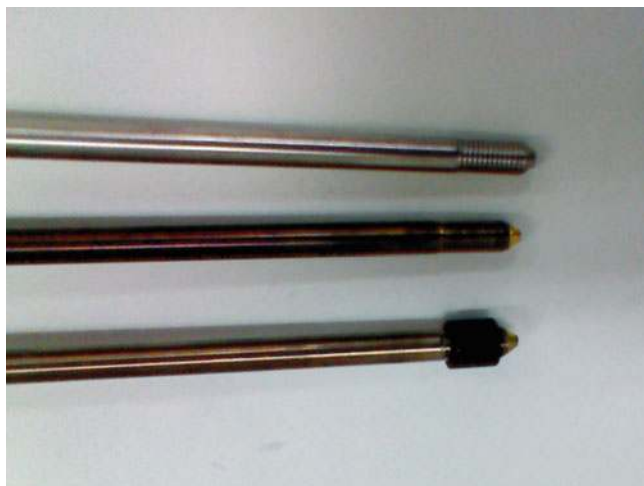
Fig. 7.3 Photo of sampling tube with gold liner
