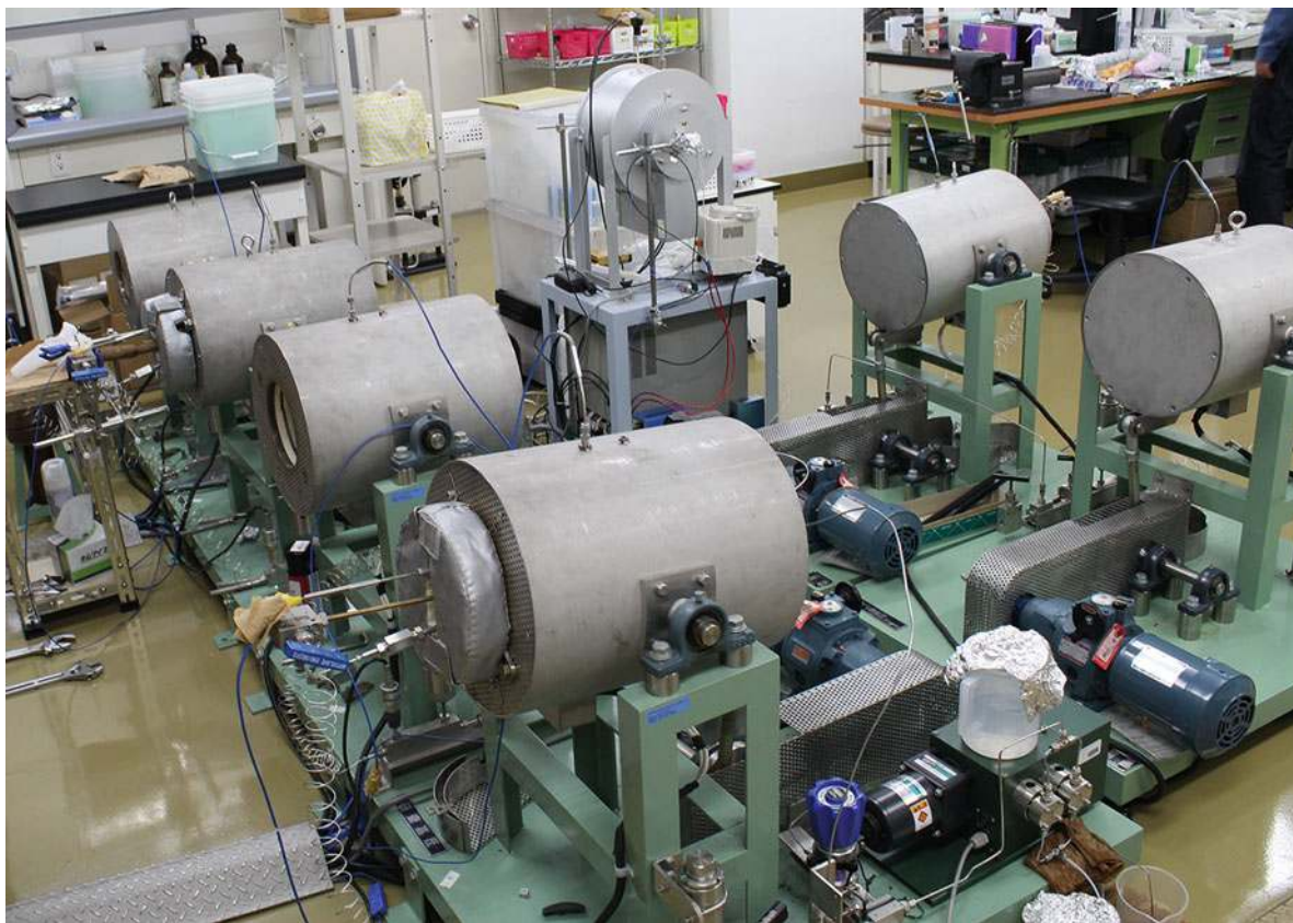
Fig. 7.1 Photo of Dickson-type autoclaves at JAMSTEC
