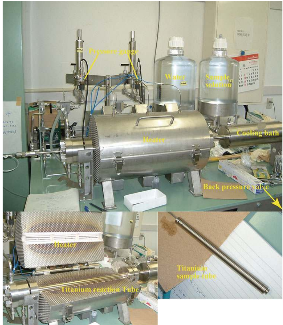
Fig. 7.5 Photos of flow-type experimental system developed at JAMSTEC for simulation of water-rock interactions
