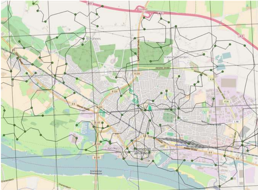
Fig. 13 Area of Emmerich with German 1 km × 1 km grid and power nodes and lines (OpenStreetMap)
