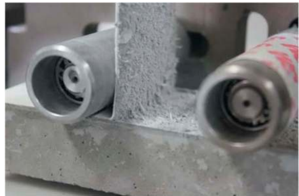
Figure 4. Strong bond between membrane and concrete.
