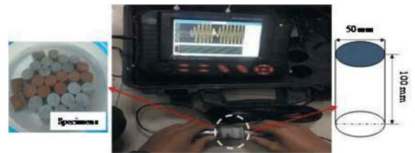
Figure 4. The test of the elastic wave velocity of rock.
