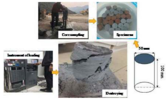
Figure 3. The test of uniaxial compressive strength and elastic modulus of rock.
