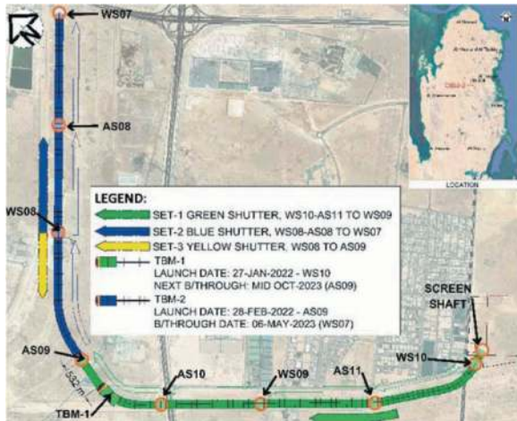
Figure 1. WWDT project layout/progress.
