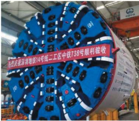
Figure 2. The first EPB-TBM dual-mode shield CREC738 applied in Shenzhen Metro.
