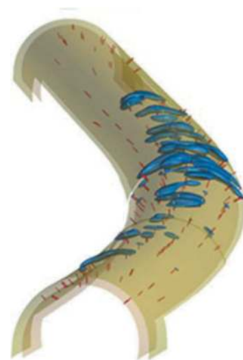
Figure 8. Voids model (Leapfrog works).
