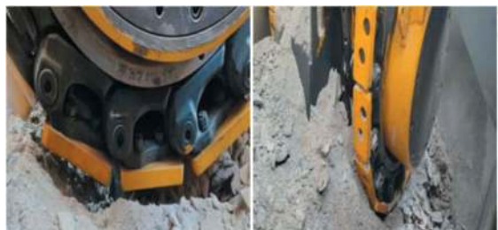
Figure 8. (a) Chain tension state (b) Filling of slag silo.
