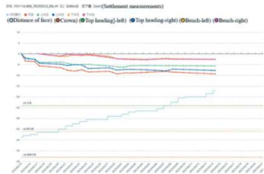
Figure 13. Results of tunnel settlement and convergence.
