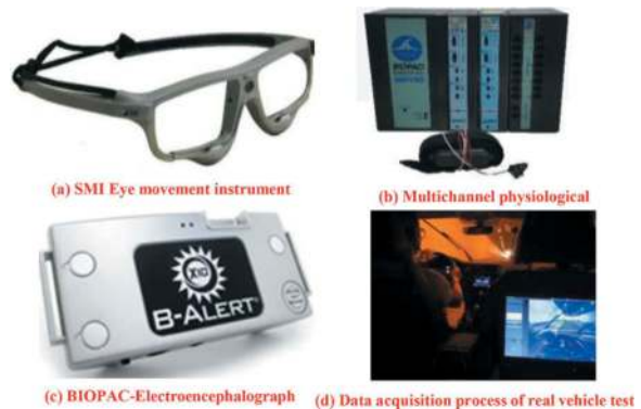
Figure 3. Collection device and acquisition process.
