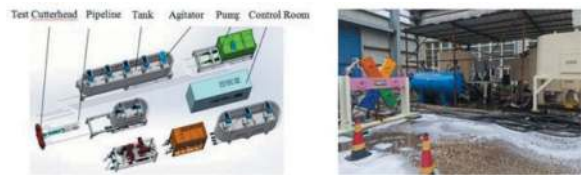
Figure 3. Composition and physical diagram of the test platform.
