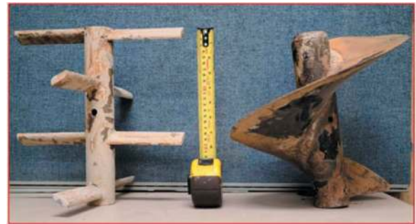
Figure 4. Impeller, Left: Pin Rotor, Right: Auger.
