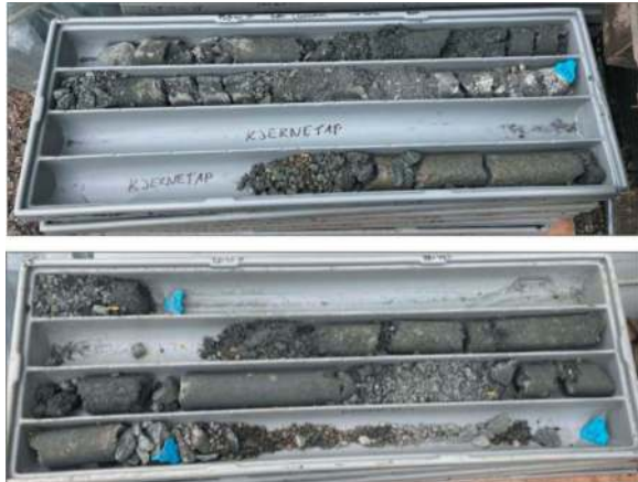
Figure 12. Retrieved core-drillings from Plan view of presumed fault zone section.
