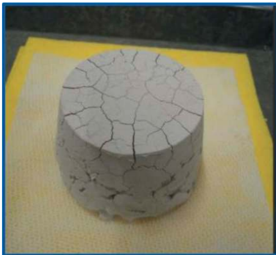
Figure 3. Conventional grout @T24hrs after 15 strokes on Hagermann flow table at room temperature.
