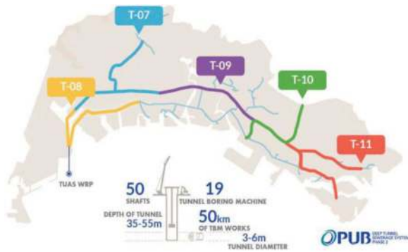
Figure 1. DTSS Phase 2 Project Layout.
