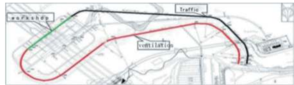
Figure 5. TBM tunneling route.
