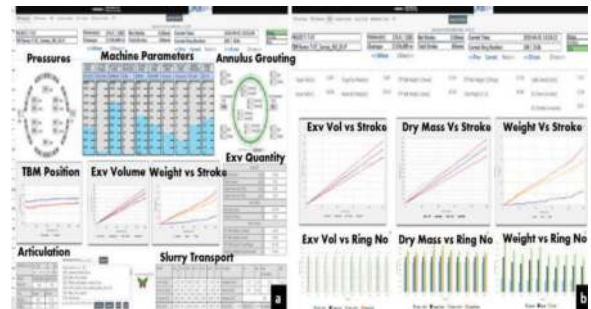
Figure 13. Real-time TBM monitoring dashboard tabs; (a) key operation parameters, (b) AEM data.
