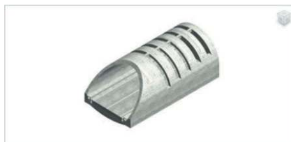
Figure 4. Hollow-cut-bamboo portal tunnel simulation model.
