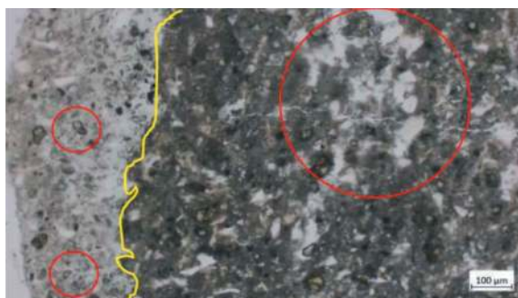
Figure 10. Detail of the passage between altered and fresh grout (yellow line). The porosity is shown in the red circles.
