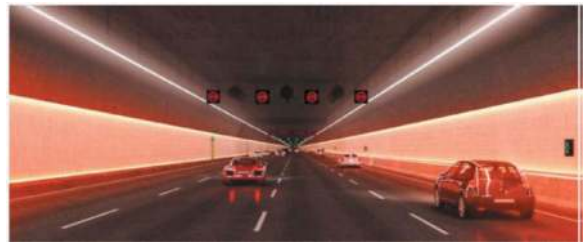
Figure 4. Diagrammatic Sketch of Side Wall Light Strip in the Tunnel.
