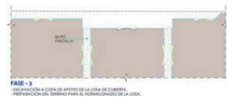
Figure 6. Phase 3 cut and cover.
