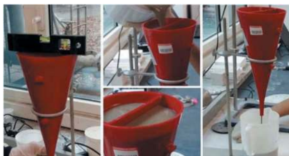
Figure 4. Marsh funnel used for the flow time assessment. (Todaro et al., 2023).
