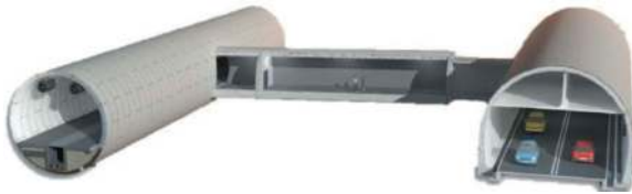
Figure 1. Fréjus road tunnel (right), new second tube (left) and a bypass (SFTRF, 2020).
