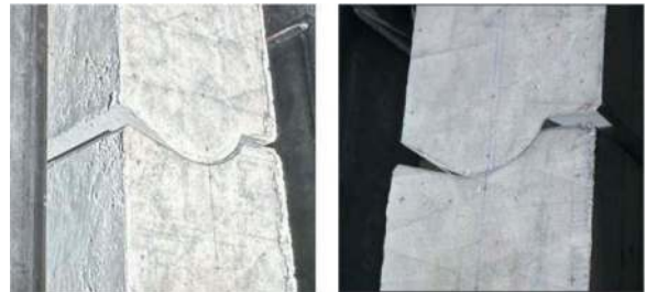
Figure 10. Test sample of case 1: no lip and twist (left) and case 2: +10mm lip and twist (right).
