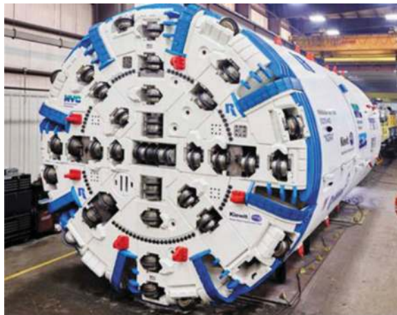
Figure 2. Hard rock TBM cutterhead central disc rotor and outer circular shell front view (6).
