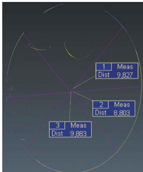
Figure 6.2. Oblique slices detected when the diameters or not equal.
