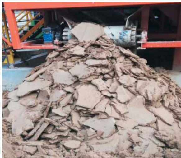
Figure 9. Filter press dewatering.
