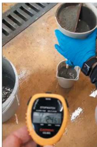
Figure 2. Flowing test with Marsh cone.
