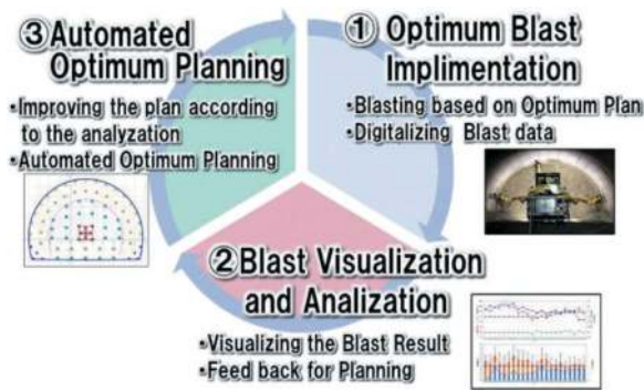
Figure 3. The positive loop for optimum blasting.
