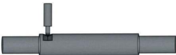
Figure 4. CFD grid model of water-gas mixing device.
