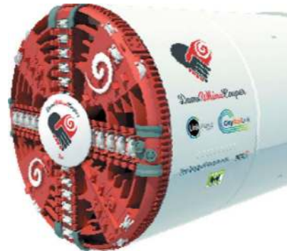
Figure 3. CRL's EPB TBM, Dame Whina Cooper.
