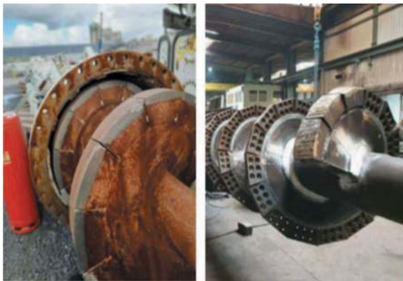
Figure 7. Screw conveyor before and after the remanufacturing process.
