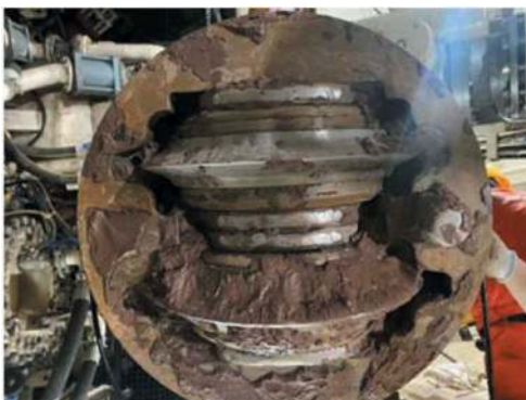
Figure 5. Tool secondary wear.
