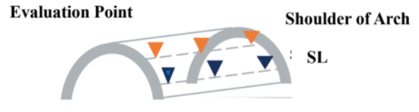
Figure 15. Location of surface water absorption test and surface air permeability measurement.
