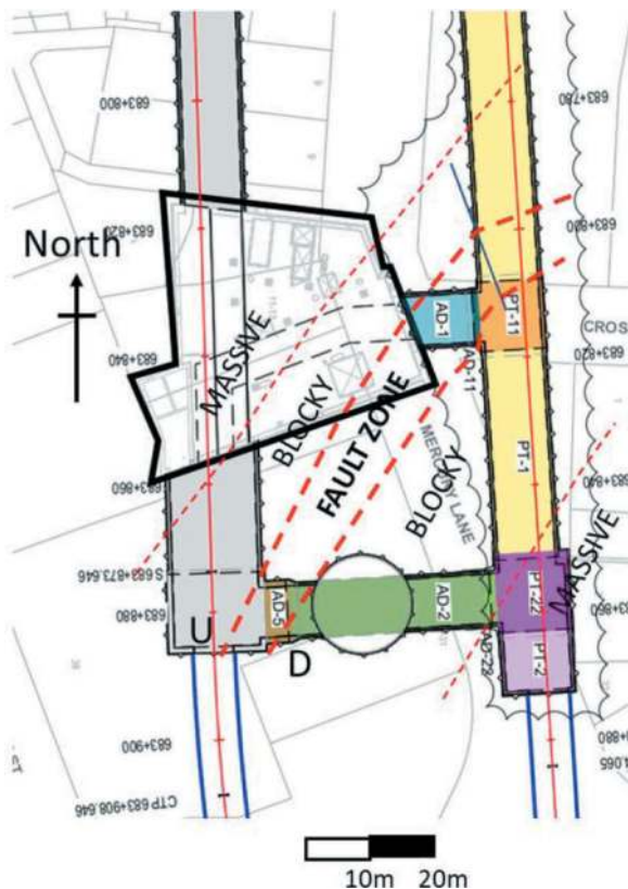
Figure 5. Mapped shear zone associated with normal faulting.
