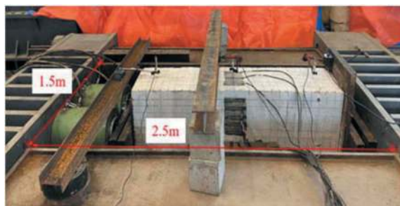
Figure 6. Homemade counterforce frame device.
