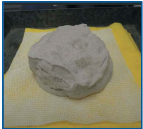
Figure 5. The new grout solution @T24hrs after 15 strokes on Hagermann flow table with improved rheology & no cracks.
