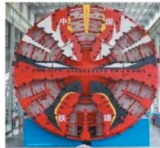
Figure 6. Jinghua: (16.07m) spatula type atmospheric pressure cutter head.
