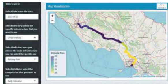
Figure 8. Example of C2RISK tool giving information about vulnerability to climate change of an Italian railway line, in terms of risk for infrastructures.
