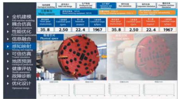
Figure 5. Operation simulation based on digital twin.
