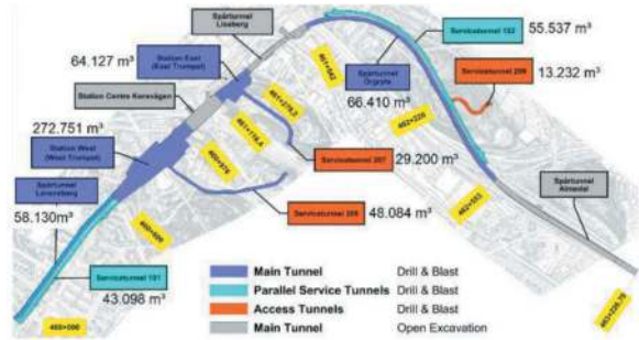
Figure 3. Main construction sections and details.
