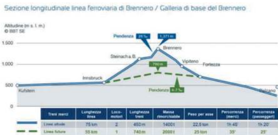
Figure 2. Comparison of the existing railway line and the future Brenner Base Tunnel.
