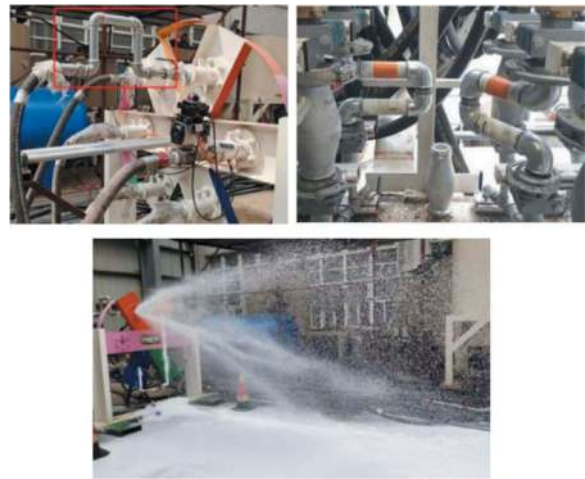
Figure 9. Foam injection test with “Ω” device.
