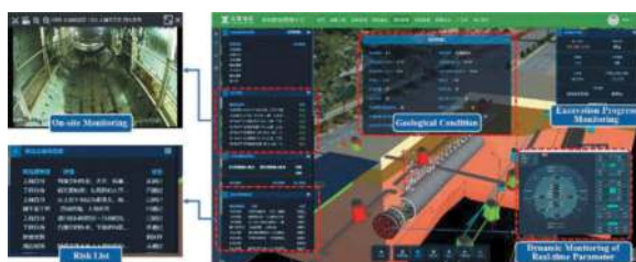
Figure 7. Fine management of shield tunnelling based on 3D space.
