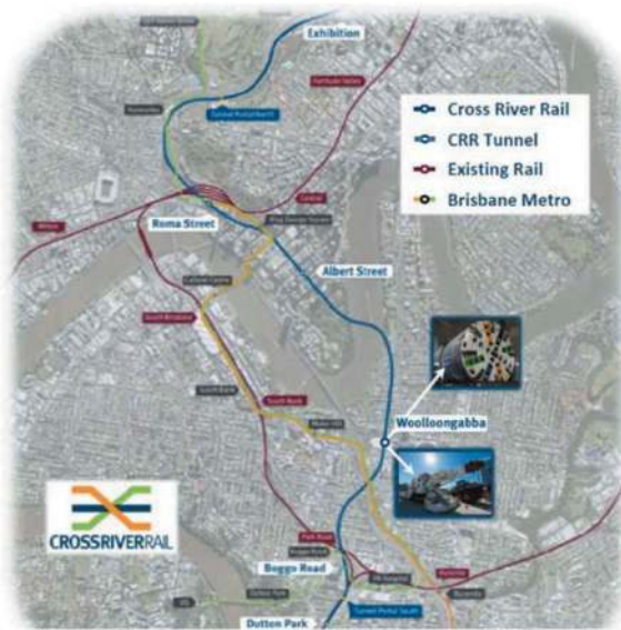
Figure 1. Overview of tunnel excavation. Roadheader tunnels from Woolloongabba to Boggo Road. TBM tunnels from Woolloongabba to Northern Portal.
