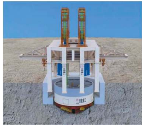
Figure 4. Full-face shaft boring machine.
