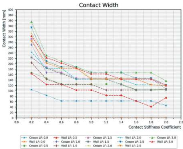
Figure 13. Variation of contact width with contact stiffness, where a load factor of 0.0 represents self-weight.
