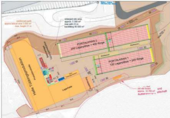
Figure 4. Plane view of tubbing factory (yellow) and tubbing storage (red) on the reinforced earth.
