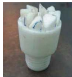
Figure 9. Plastic drilling bit.
