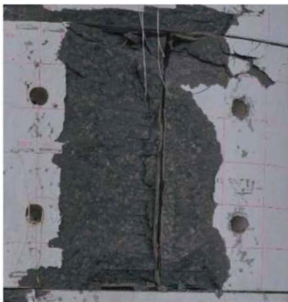
Figure 4. Ultimate failure state of tested segment (Liu et al., 2017).
