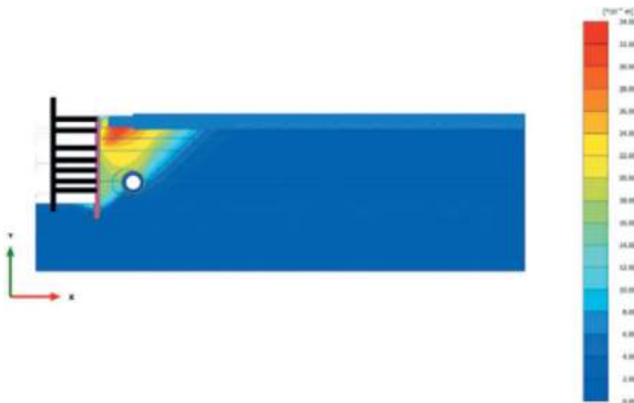
Figure 11. Maximum Total displacement near ground surface after final level excavation of cut & cover Box: 32mm.
