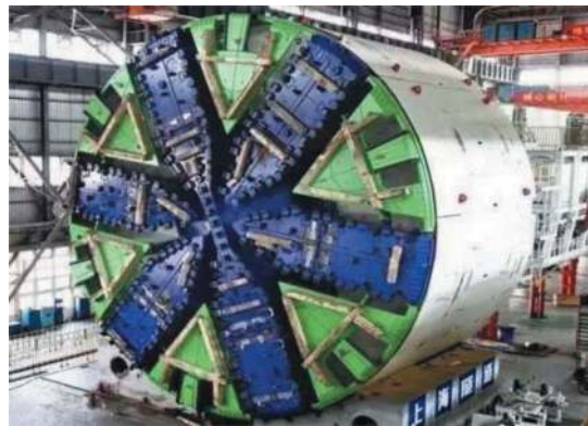
Figure 4. The TBM used in BEP II.
