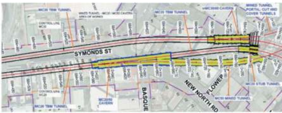
Figure 2. Maungawhau Mined Tunnel layout.
