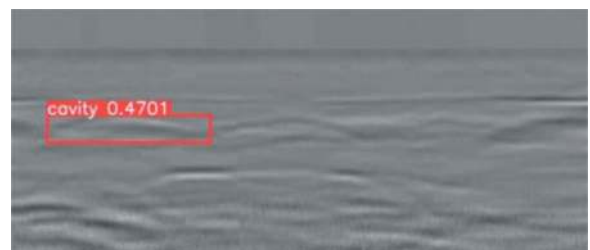
Figure 12. Cavity bounding box and accuracy results in a real-world GPR image for detection Model C.
