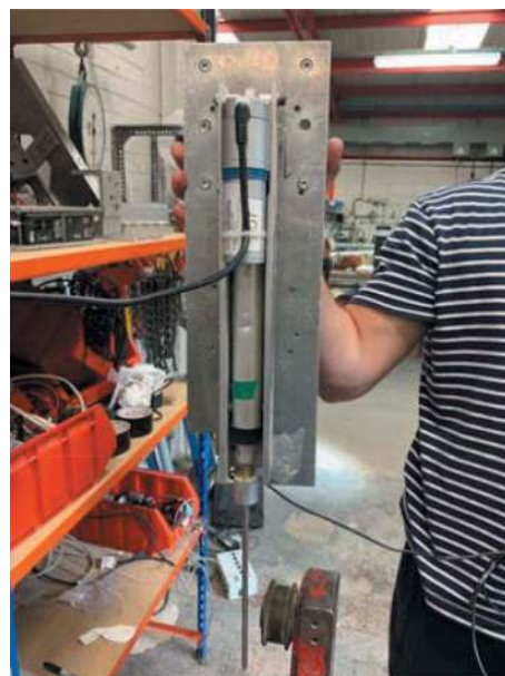
Figure 3. CPT system adopted in test ZA04.
