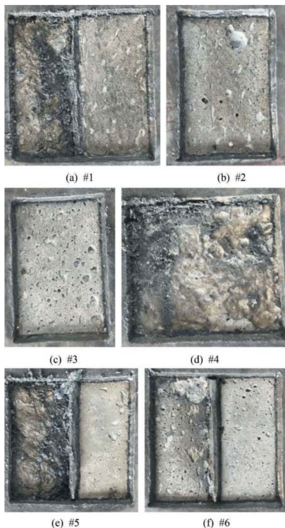
Figure 7. Opening condition of steel case Nos. #1 to #6.
