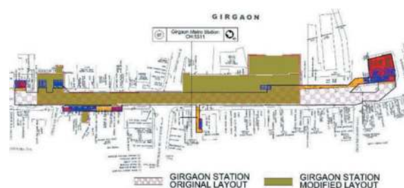
Figure 3. Original & modified layout of Girgaon Metro Station.
