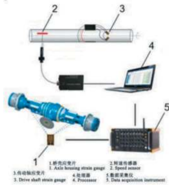
Figure 7. Schematic diagram of acquisition system construction.
