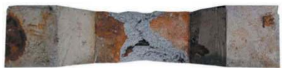
(c) The failure mode of the C-side
