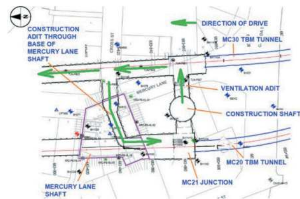
Figure 7. Construction access for MC21.
