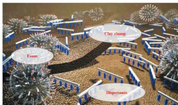
Figure 5. Schematic diagram of the mechanism of dispersants.
