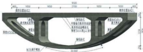
Figure 3. Detail of the prefabricate arc parts.
