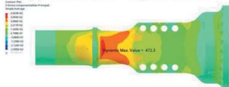
(2) Vertical force Fz + lateral bending moment Fmy (14°)
