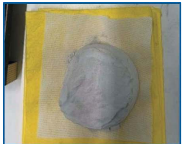
Figure 6. The new grout solution @T28days at room temperature with improved durability, no segregation.
