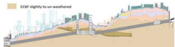
Figure 5. Longitudinal geological section of the bored tunnels.
