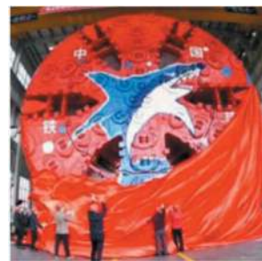
Figure 7. Tuodao: (13.42m) hob and scraper combined type atmospheric pressure cutter head.
