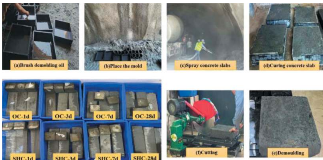
Figure 1. The forming process of shotcrete slab and soaking process.
