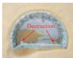
Figure 13. Deformed tunnel model of Case 4.
