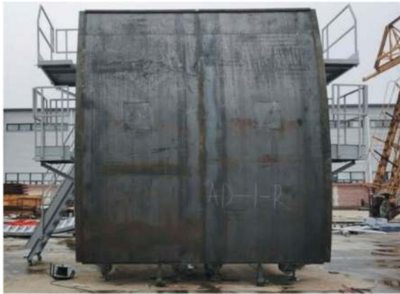
Figure 13. 4m Sidewall Formwork.
