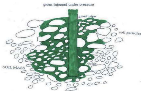
Figure 3. Schematic sketch of the TAM technique.
