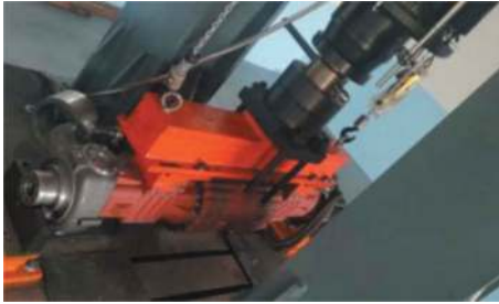
Figure 8. Loading platform for load calibration.
