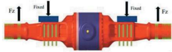
Figure 2. Schematic diagram for application of vertical load ( F_z ).
