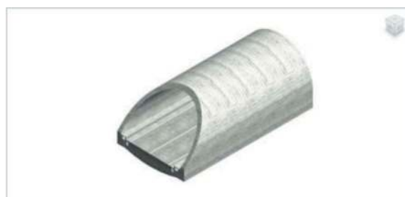
Figure 3. Cut-bamboo portal tunnel simulation model.
