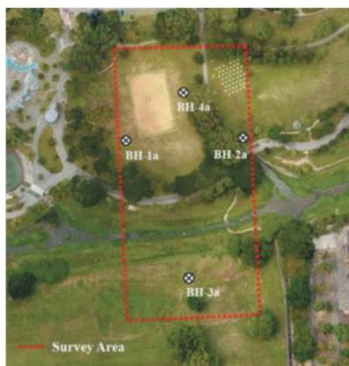
Figure 1. Survey boundaries and borehole layout at Bishan Park.
