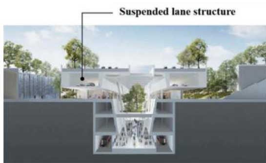
Figure 6. Suspended lane structure.
