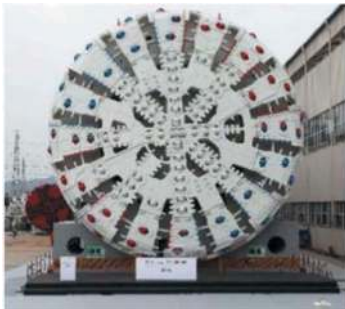
Figure 3. 14.2m diameter TBM (S882) in the Nansha factory.
