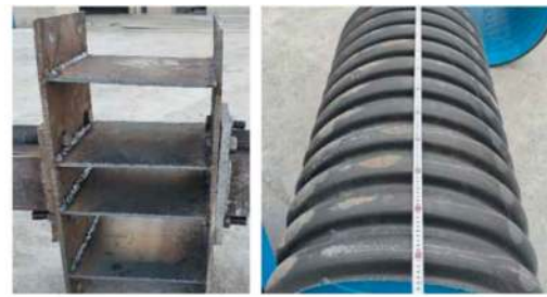
a) Hoop flexible components b) Radial flexible components
