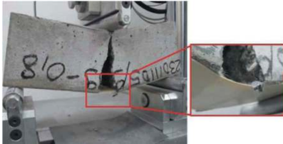
Figure 5. Crack bridging test.
