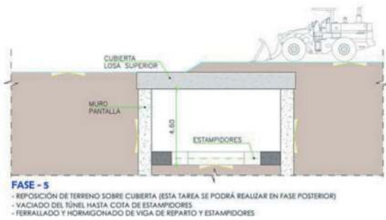
Figure 8. Phase 5 cut and cover.
