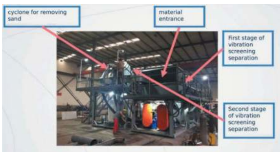
Figure 7. The separation equipment of sand and mud.
