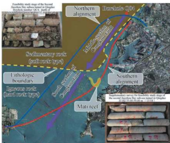
Figure 2. Tunnel address scheme in Jiaozhou Bay.
