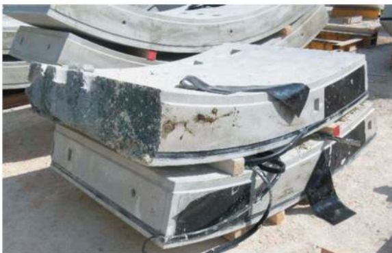
Figure 3. Detail of another halved SFRC segment (both pieces).
