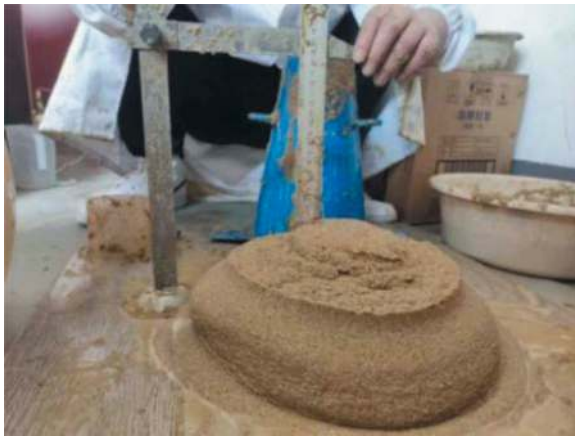
Figure 3. Conditioned soil with a slump of 125mm.
