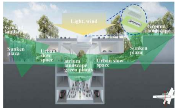
Figure 17. Schematic diagram of “bringing the wind into the city” of Huangmugang Hub.
