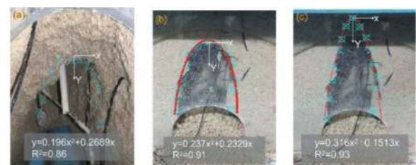
Figure 2. The fitting curves of the collapse arches. a. The first collapse arch; b. The second collapse arch; c. The third collapse arch.
