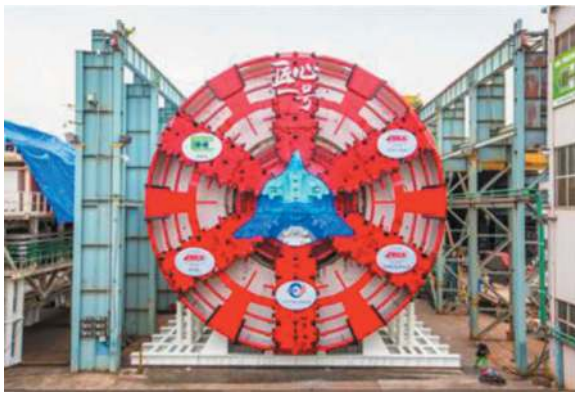
Figure 3. Cutting wheel for the right line tunnel of Jiangyin Jingjiang Yangtze River Tunnel.
