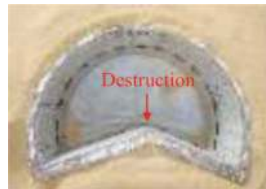
Figure 9. Deformed tunnel model case 2.
