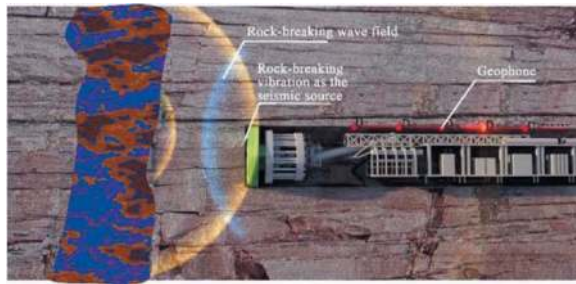
Figure 9. Geological Prediction with rock-breaking vibration as the seismic source.
