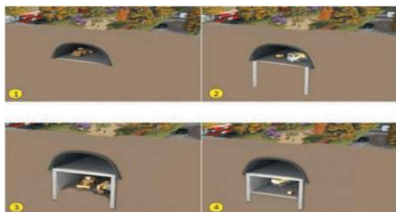
Figure 7. Hybrid tunnel construction sequence.
