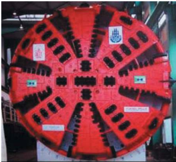
Figure 2. A view of the cutterhead of TBM used.
