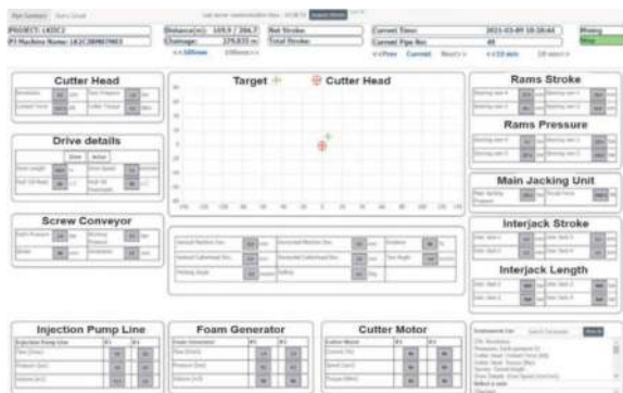
Figure 15. Pipe jacking monitoring dashboard.
