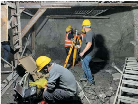
Figure 9. Photos of drilling radar on-site testing.
