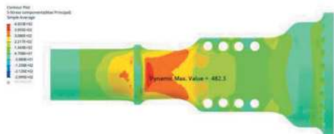
(2) Vertical force Fz + lateral bending moment My (14°) + lateral tension Fyl
