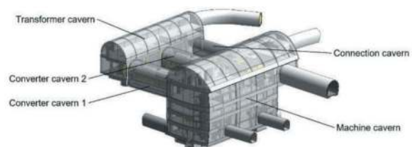
Figure 4. Double cavern solution.
