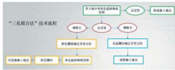
Figure 10. Technical process of “three hole combination method”.
