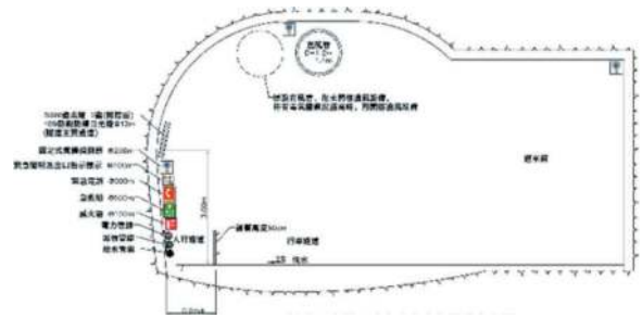
Figure 7. Location of the automatic gas detector.
