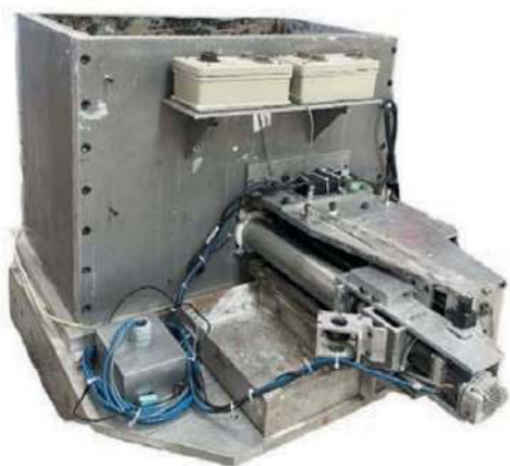
Figure 2. Model TBM system attached to tunnelling box.
