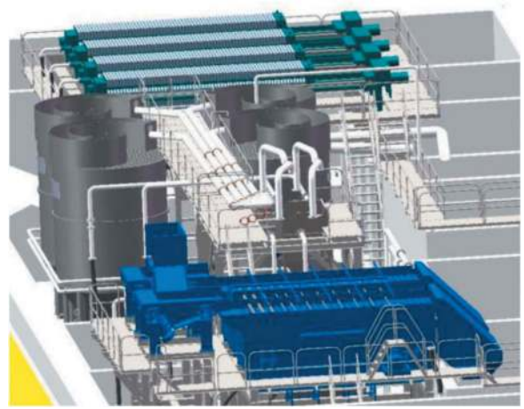
Figure 11. BIM modeling of shield tunneling slag treatment equipment.
