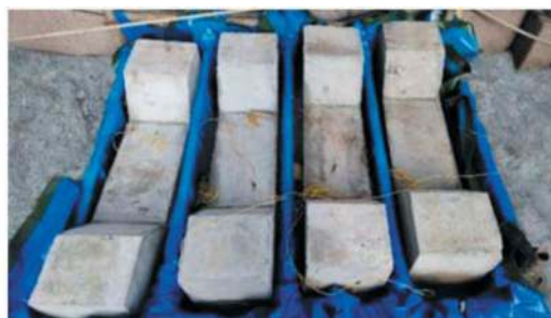
(a) Outdoor accelerated electrolytic corrosion test
