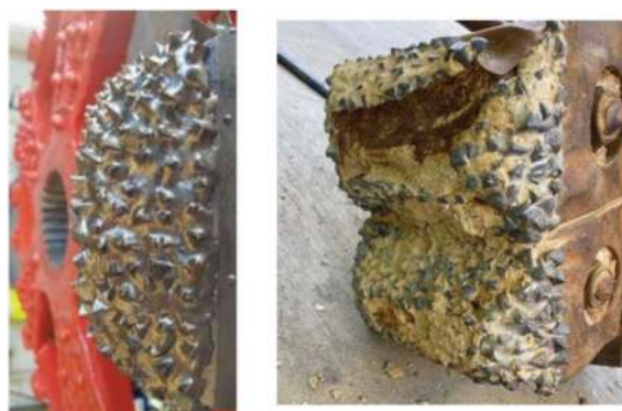
Figure 4. PVD cutting tools – fresh cutters (left), worn cutters (right).
