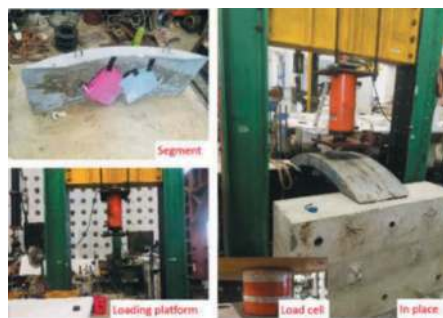
Figure 9. The set-up for loading test.
