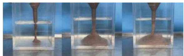
Figure 9. Underwater anti-dispersion mud slurry filler for underwater casting.
