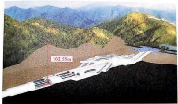
Figure 4. Perspective view of Badaling underground station.
