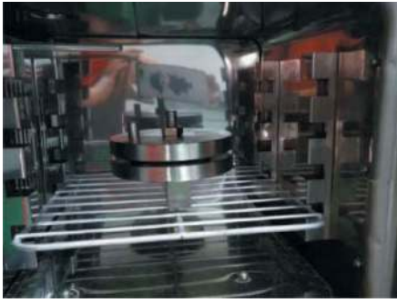
Figure 5. Electronic universal tester for compression test.
