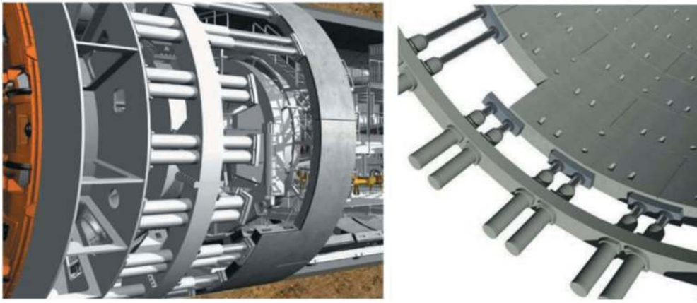
Figure 1. Illustration of TBM thrust jacking loads applied to ring end/bearing area of most recently installed segments. (left: Herrenknecht, 2015, right: Groeneweg 2007).
