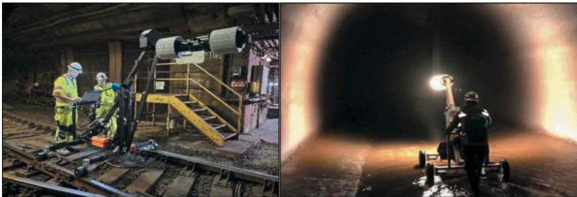
Figure 5. Altira System in subway tunnels on the left and in a water tunnel on the right. The measuring system is supported by a robust aluminum construction with a specially designed rail/wheel cart. Altira consists of an LED flash-lighting unit (white), cameras, and the LiDAR scanner (gray puck).
