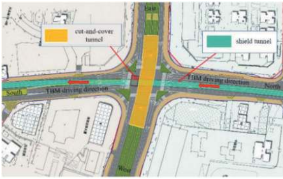
Figure 1. Floor plan of the undercrossing construction.
