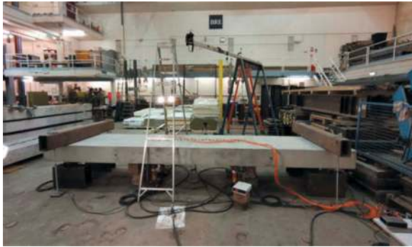
Figure 7. Laboratory beam test set-up.
