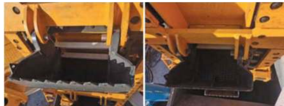
Figure 7. (a) Conventional slag bucket (b) Water-carrying slag bucket.
