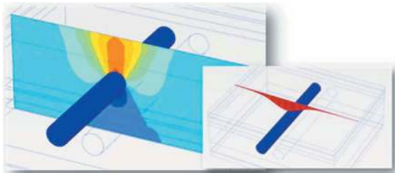
Figure 6. Settlement after one tunnel excavation.
