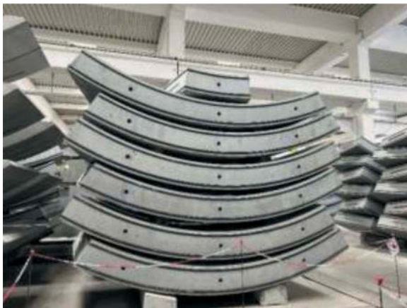
Figure 13. 6+1 prefabricated segments forming a ring.
