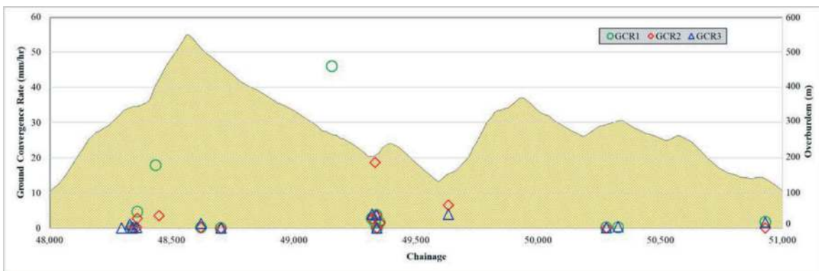
Figure 13. Ground convergence rates using data obtained from void measurement cylinders during TBM stoppages.
