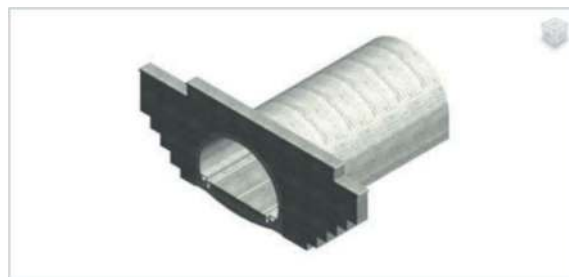
Figure 2. End-wall portal tunnel simulation model.
