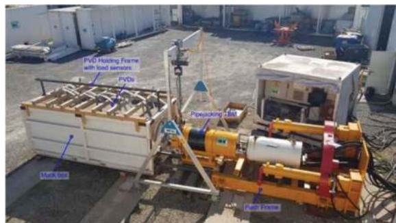
Figure 3. PVD cutting trial setup.
