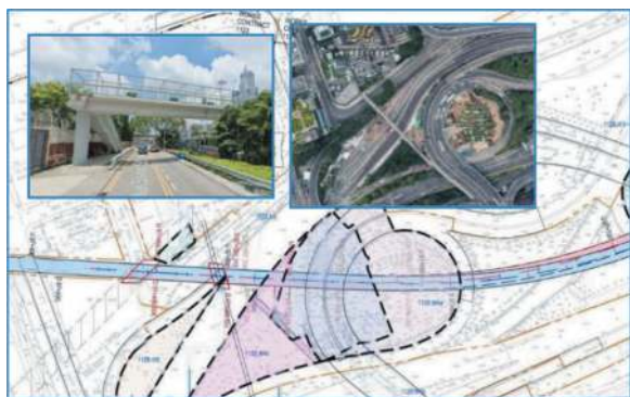
Figure 6. Major pile obstructions below Canal Road Flyover and Wan Shing Street Footbridge.
