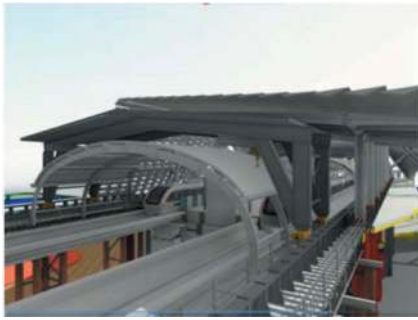
Figure 17. Schematic diagram of the mobile protective shed of the Dayun hub.
