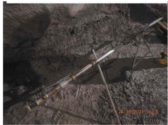
Figure 11. Optical Borehole Imager (OBI).
