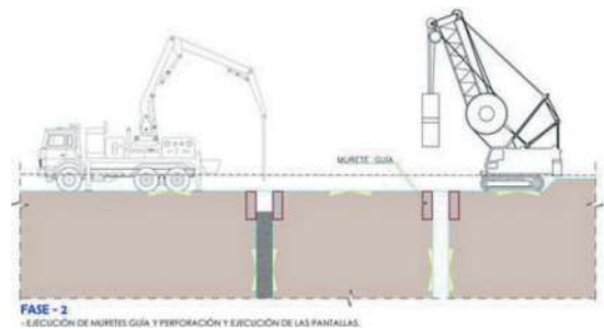
Figure 5. Phase 2 cut and cover.
