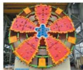
(b) Changde Yuanjiang Crossing River Tunnel shield machine cutter head
