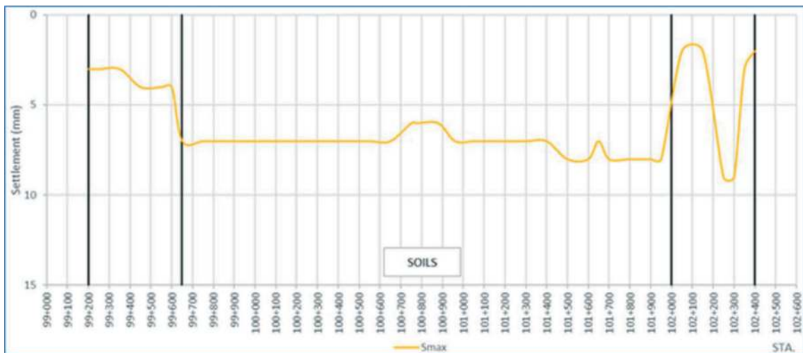
Figure 12. Settlement due to tunnel construction in soils and mix-face conditions.
