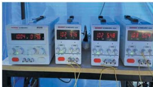
(b) DC power supply equipment
