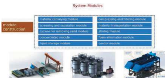
Figure 10. Main module construction.
