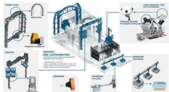
Figure 2. ARCHITA configuration for rail inspection, equipped with tunnel scan, lights, georadar, thermal imaging cameras.
