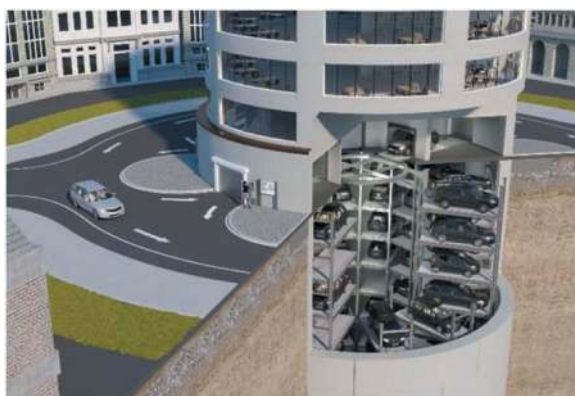
Figure 7. Exemplary use of the U-Park ® as foundation structure.
