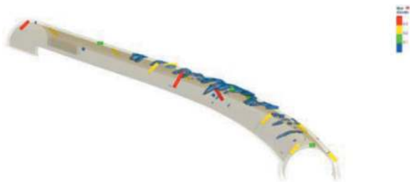
Figure 9. Flat jacks and voids model (Leapfrog works).
