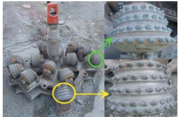
Figure 1. Reamerhead, four and five rows cutters of Sandvik Rhino 1088DC RBM.
