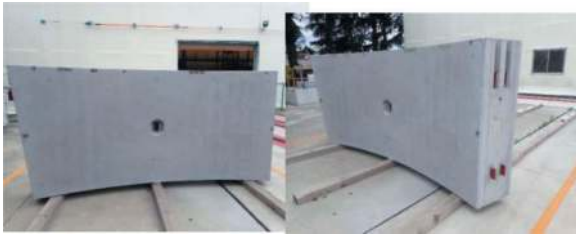
Figure 7. Concrete segment for road tunnel TBM.
