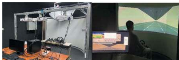
Figure 4. Dynamic information perception simulation testing platform.
