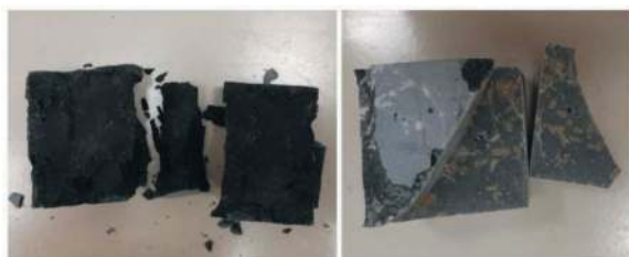
Figure 9. Pictures of samples retrieved from the full-scale block. On the left a sample taken far from the drainage hole, on the right one taken close to it.
