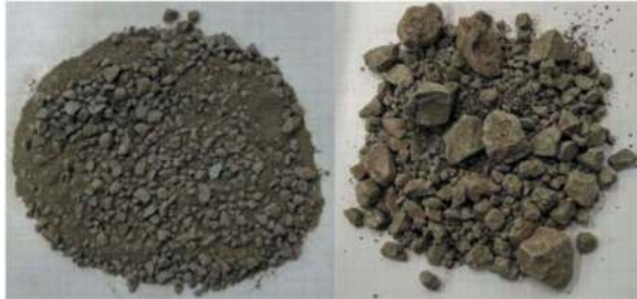
Figure 2. Clay samples used in the laboratory for the test campaign. DCC (left) e NCC (right). The difference in color is due to the different water content in the samples.
