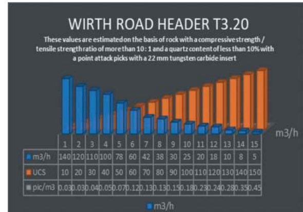
Figure 6. Road header's performance parameters by manufacturer.
