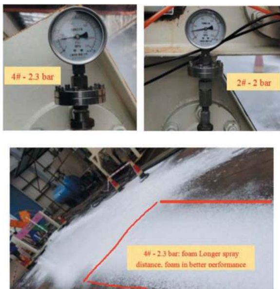
Figure 10. Comparative test on foaming effect of different distance between foam generator and nozzle.
