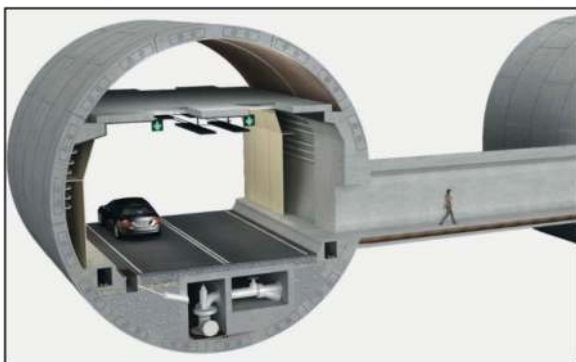
Figure 9. Cross passage between two TBM tunnels.
