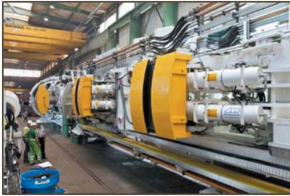
Figure 4. A view of gripper TBM.
