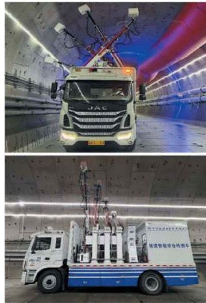
Figure 15. On-site operation of TBM tunnel structure detection.
