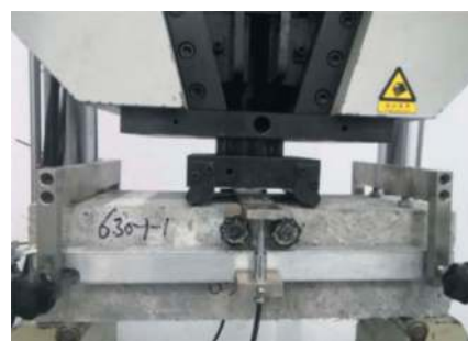
Figure 1. Beam specimen and deflection test sensors.
