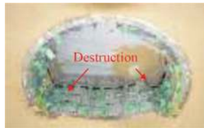
Figure 7. Deformed tunnel model of case 1.
