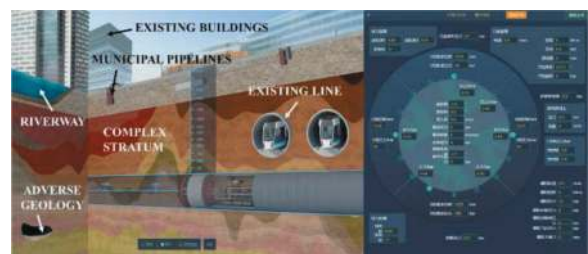
Figure 3. 3D space of shield tunnelling construction.
