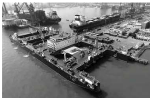
Figure 32. Transport & installation integrated vessel for Shenzhen-Zhongshan Link (Chen Hong, at el. 2022).
