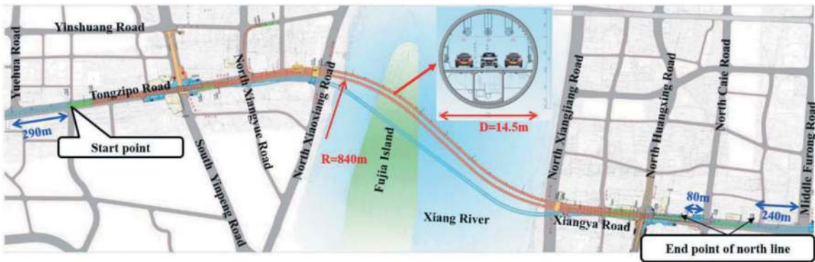
Figure 2. The overall layout of the Xiangya Road River-crossing Tunnel and the section of the shield tunnel.
