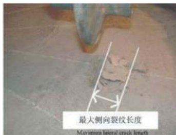
Figure 9. Hob indentation experiment.
