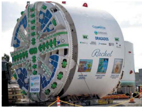
Figure 2. Mixshield TBM “Rachel” being assembled at the Carson launch shaft.
