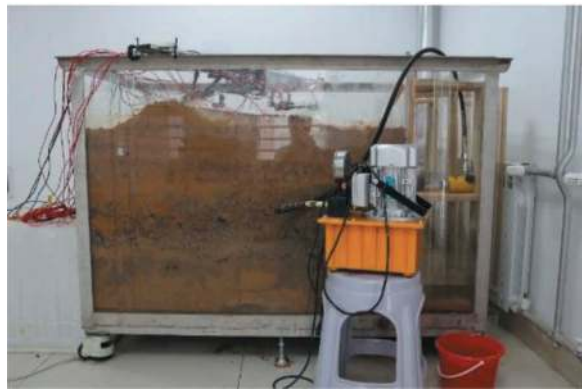
Figure 3. Model testing device.
