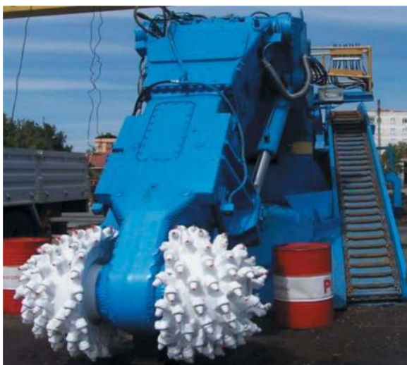
Figure 3. Transverse type roadheader used in the project.
