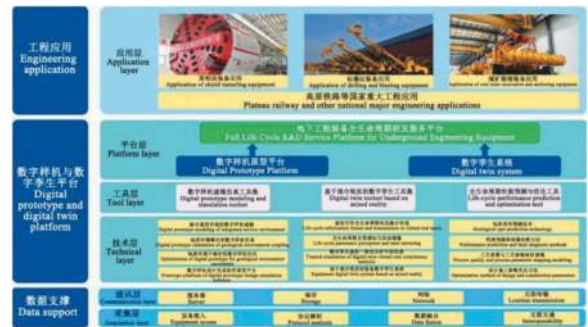
Figure 10. Implementation framework of digital twin technology for underground engineering equipment.
