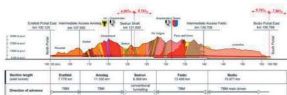
Figure 2. Geological profile of the Gotthard Base Tunnel, with localisation of the Sedrun Shaft (Source: Tunnelling the Gotthard , STS Tunnelling Society, 2016).
