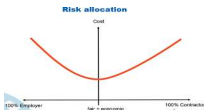
Figure 3. Conceptual evolution of project costs depending on risk allocation to the Contractor.
