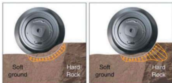
Figure 7. Schematic illustration of the forces acting on a cutting disc at a mixed face tunnel.
