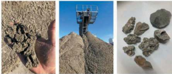
Figure 5. Pictures of the muck (sand; shell fragments).
