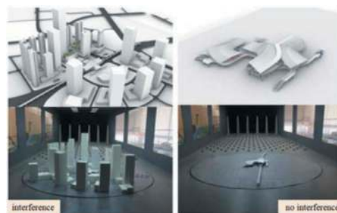
Figure 14. Wind tunnel test.
