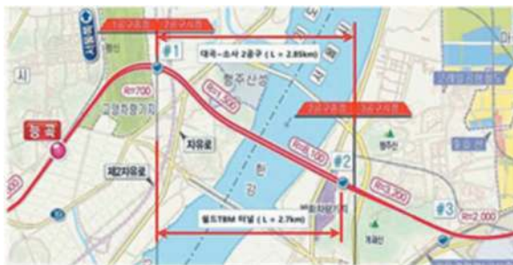
Figure 1. Construction plan overview.
