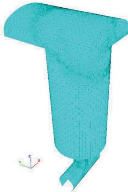
Figure 3. Finite element model (FEM) of surge tank.
