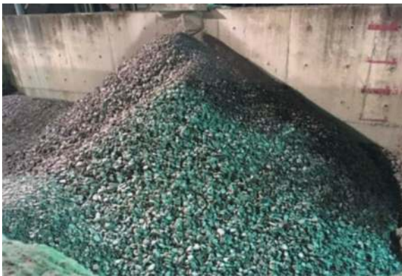
Figure 10. Muck Pit for gravel.
