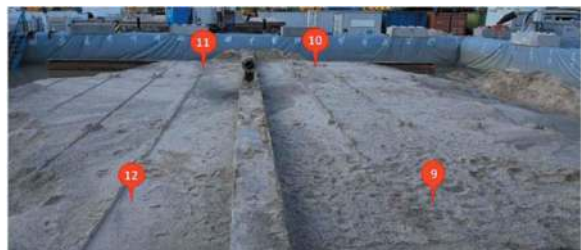
Figure 8. Result of Sand flow test with Kaliwaal 41.
