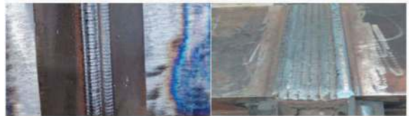
Figure 12. Multi-layer and Multi-pass Weld Seam Results.
