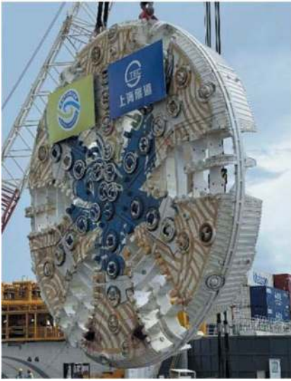
Figure 5. Shield cutterhead and disc cutter.
