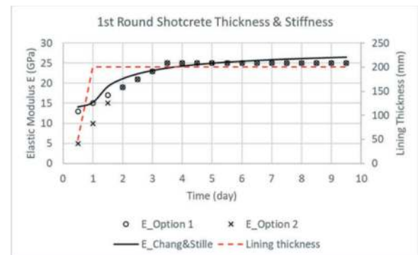
Figure 12. Shotcrete lining thicknesses and stiffness.
