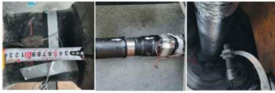
a) Axle housing strain gauge b) Drive shaft torque strain gauge c) Drive shaft speed sensor
