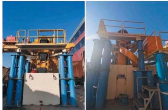
Figure 6. (a) Bucket surface of vertical slag removing machine (b) Slag chute surface.
