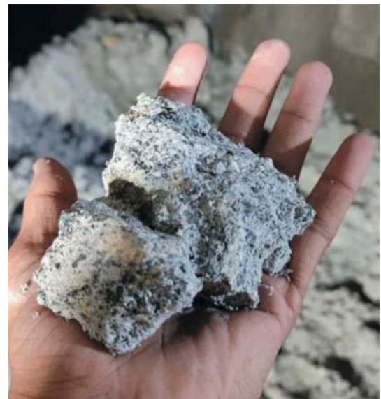
Figure 8. Crushed dolomite mixed with PU-2C grout.
