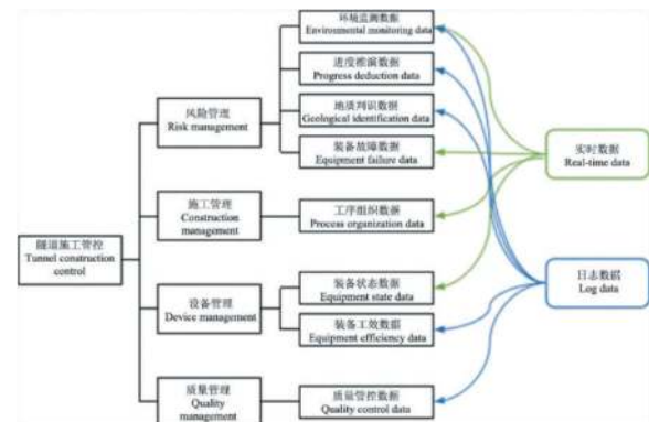
Figure 1. Classification of data about tunnel construction control.
