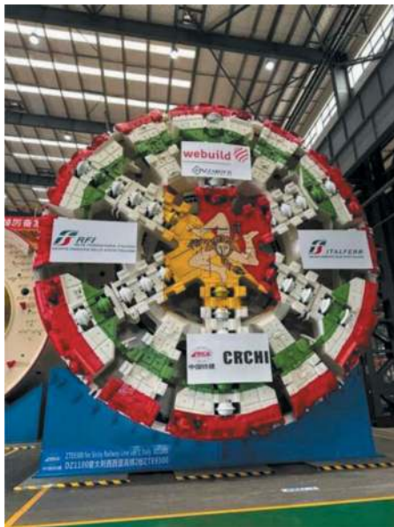
Figure 3. The first CRCHI EPB TBM for the project.
