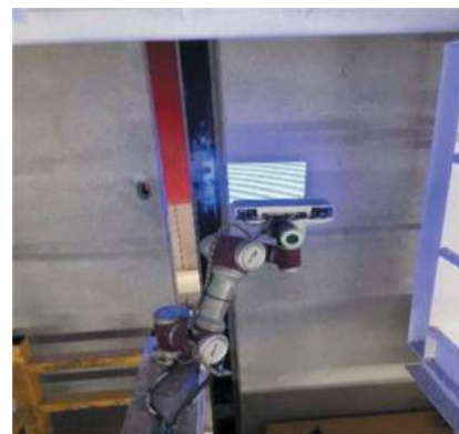
Figure 19. Upper active vision camera and structured light generator in working.
