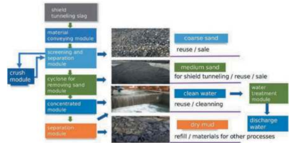
Figure 4. Schematic diagram of slag treatment process.
