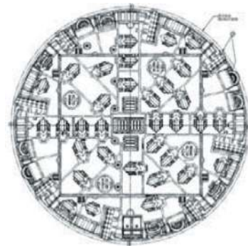
Figure 5. Schematic diagram of tool layout.
