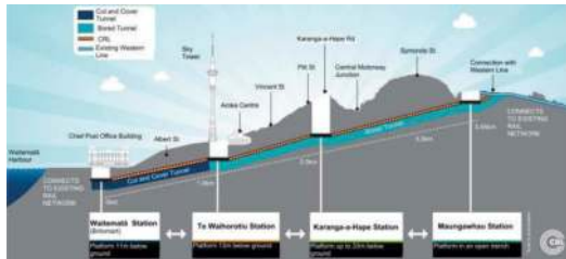
Figure 2. Section of CRL's alignment.
