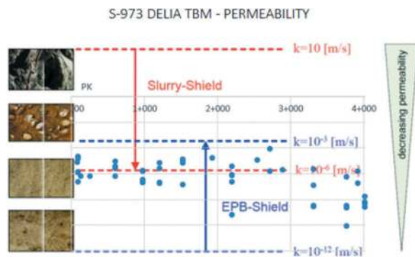
Figure 6. Ground permeability from E04 to PV01bis.
