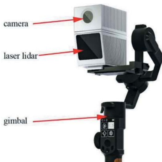
Figure 1. Equipment for collecting data.
