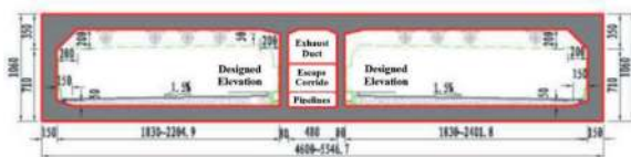
Figure 2. Cross-section of the element tubes.
