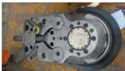
Figure 13. New cutter disc fixation (Bouygues's patent).
