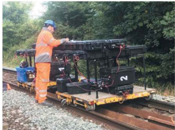
Figure 6. Image of two muon systems on railway tracks.
