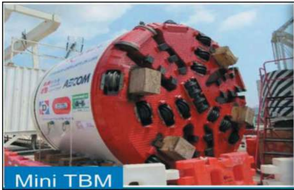
Figure 12. Mini-TBM (OD 3.665m) for cross passage construction.
