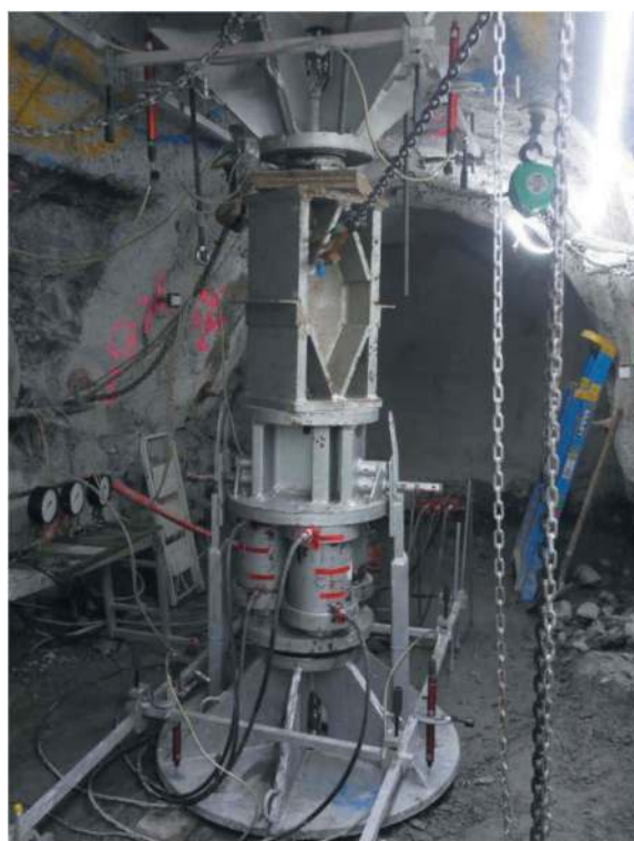
Figure 15. In-situ plate load test.
