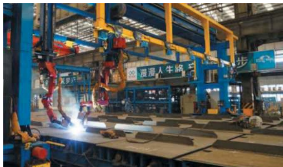
Figure 11. Application of sheet body intelligent welding in steel shell and ship products.
