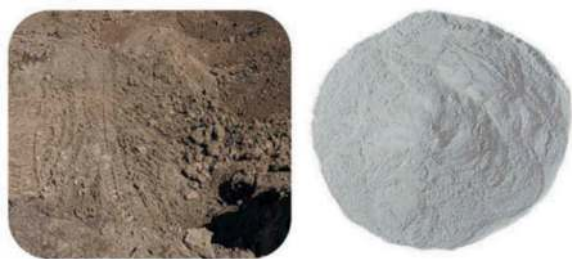
Figure 6. Base material, Left: Denver clay, Right: Wyoming Bentonite.
