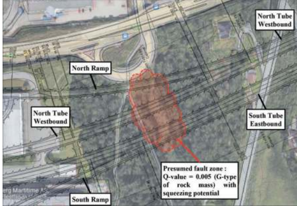
Figure 11. Plan view of presumed fault zone section.
