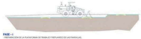
Figure 4. Phase 1 cut and cover.
