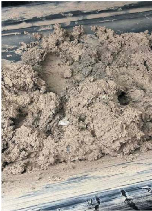
Figure 3. Conditioned soil southbound drive.
