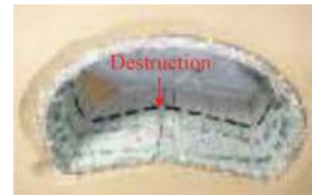
Figure 11. Deformed tunnel model of case 3.
