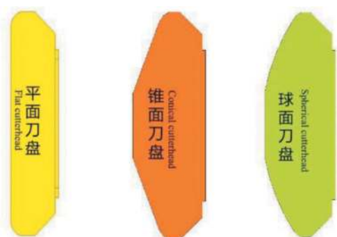
Figure 2. Schematic diagram of cutterhead structure.
