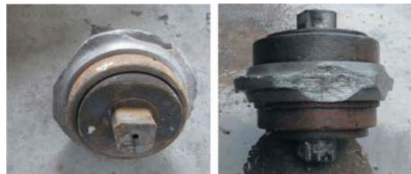
Figure 6. Abnormal wear of tool.
