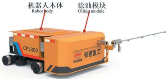
Figure 6. Quick change diagram of operation module of wall-climbing robot.
