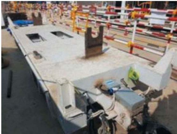
Figure 17. Flat car equipped with load cells for OBMWS.
