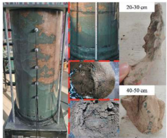
Figure 7. Grout diffusion in clay.
