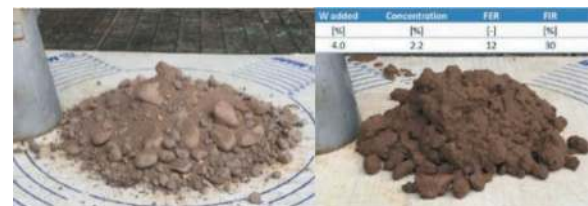
Figure 14. Sample of gravel with sand, clay, and silt before (left) and after conditioning (right).
