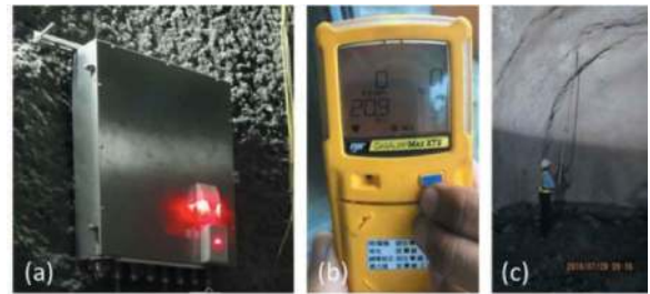
Figure 8. Site photographs: (a) fixed gas detector, (b) portable gas detector and (c) gas measurement.
