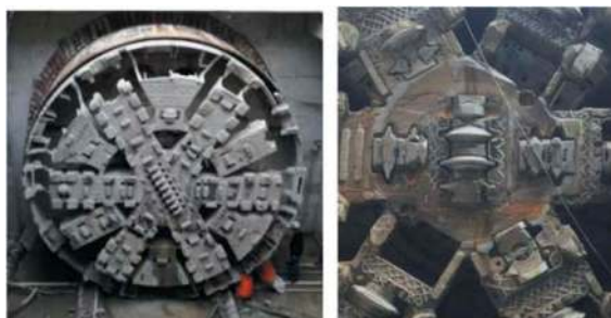
Figure 8. Damage of conventional cutter head of shield tunnelling machine.
