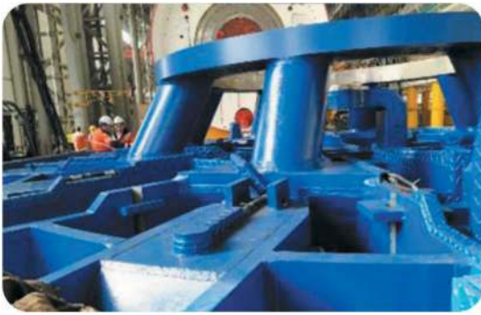
Figure 9. Ovoidal thrust rams to reduce friction.
