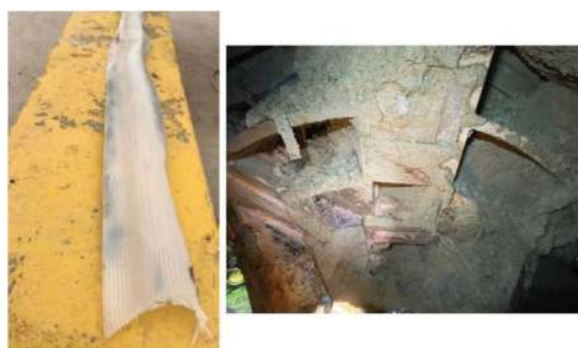
Figure 5. PVD encountered during tunnelling.
