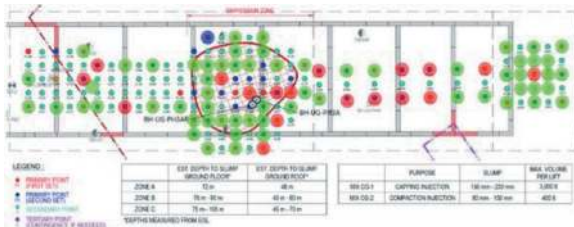
Figure 15. Compaction grouting points.
