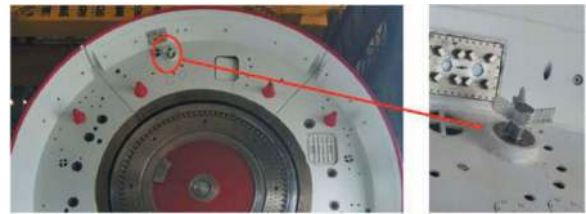
Figure 6. Void detection system (photo on CREG courtesy)
