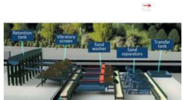
Figure 10. The arrangement of sifting facilities.
