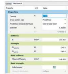
(c) Plaxis 2D cable bolts (fully bonded)
