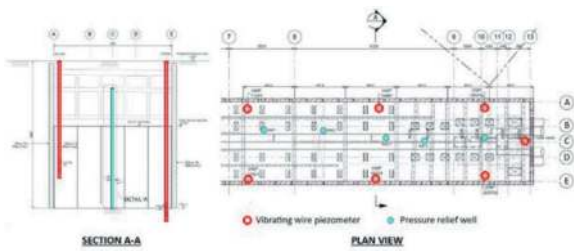
Figure 17. Provision of piezometers and pressure relief wells.
