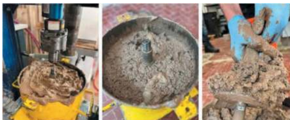
Figure 15. Dynamic adhesion test ID 1. Material completely poured into the steel container (left), material at the end of the test (right), extraction and visual analysis of the disc (right).
