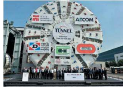
Figure 4. 17.6m diameter TBM (S880).
