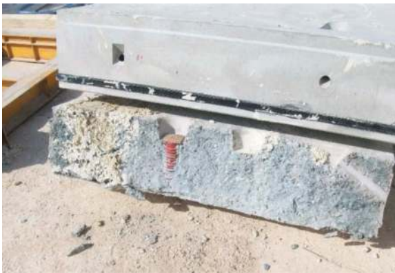
Figure 13. View of a segment split along the minor axis of the piece. The brown stain on the left is dirt from when it fell.
