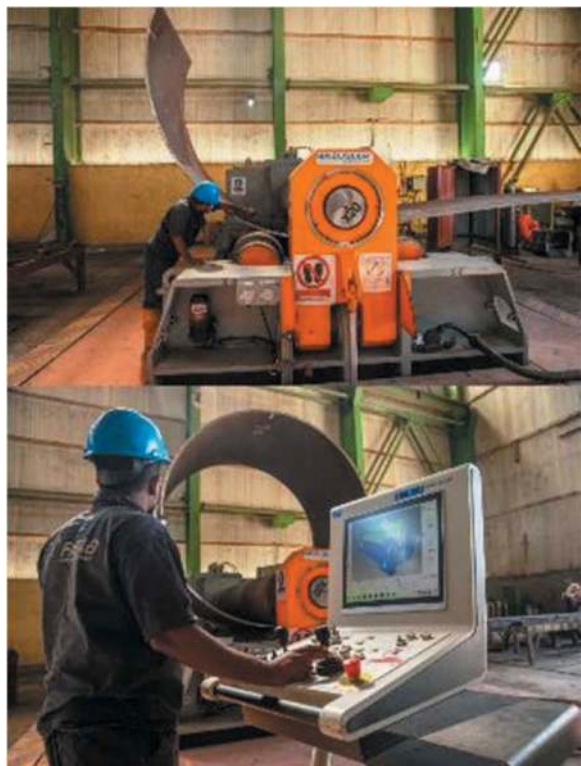
Figure 3. Rolling the steel plates for steel lining support.
