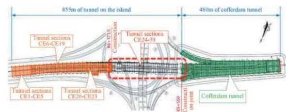
Figure 5. Schematic diagram of overall construction process of the tunnel on the Eastern Artificial Island and cofferdam tunnel.
