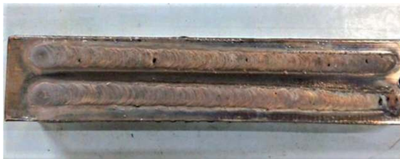
Figure 4. Cu-Sn alloy surface modified with Ni.
