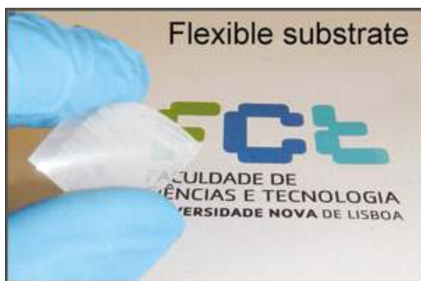
Figure 6. Photograph of TiO 2 nanostructured arrays on PEN substrates. All solvents produced similar samples, such as the one presented in this image.
