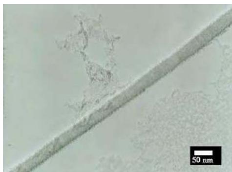
Fig. 3. TEM image of the GaNWs revealing a uniform diameter of ~40 nm.
