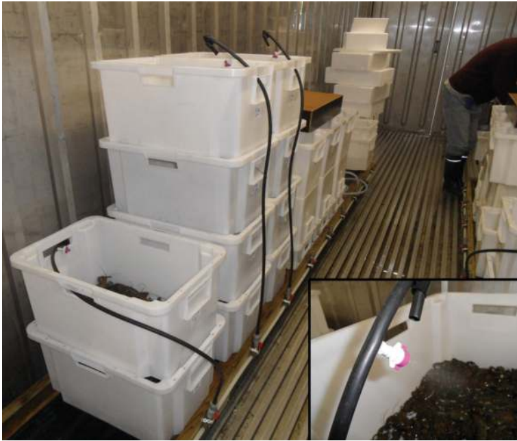
Figure 6. CrayShower with stacked plastic containers for holding of crayfish and a close-up of the water sprinkler system (small picture).
