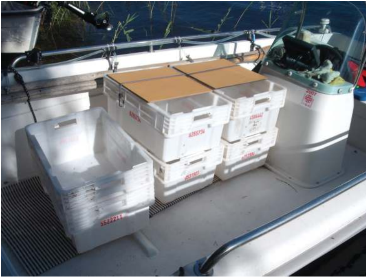
Figure 5. CrayShower on board transport application. This system uses lake surface water, thus not suitable during warmest summer days.
