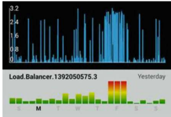
Fig. 12.3 An anomalous pattern detected within a noisy metric stream from a load balancer (picture from [109])
