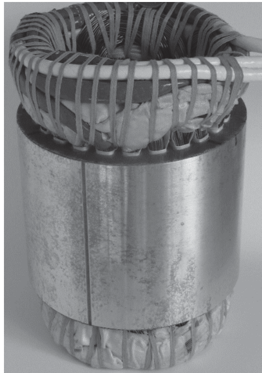
Figure 2. Electric motor end-windings wound with loose round wires.
