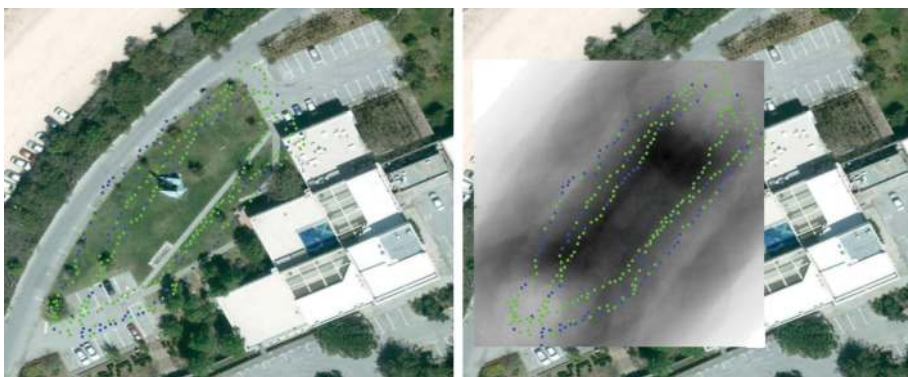
Figure 8. A heat map algorithm: No active jammer. Left: All samples. Right: The brightest regions of heat map are at the upper left and lower right corners. Since no jammer exists, the algorithm assumes it is outside the ROI.
