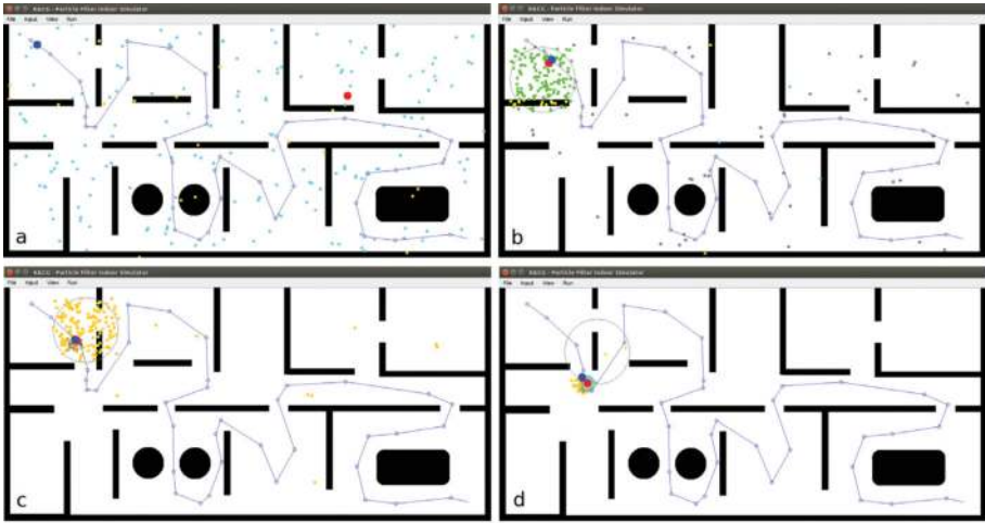
Figure 4. Particle filter in action: 100 particles were randomly located in the building (a), a WiFi positioning service was used for fast converges (b and c). All the particles converged to the correct position (d).
