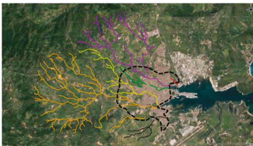
Figure 3. Creeks draining to the Olbia city center. Dashed line marks the study area where flood simulation has been conducted.
