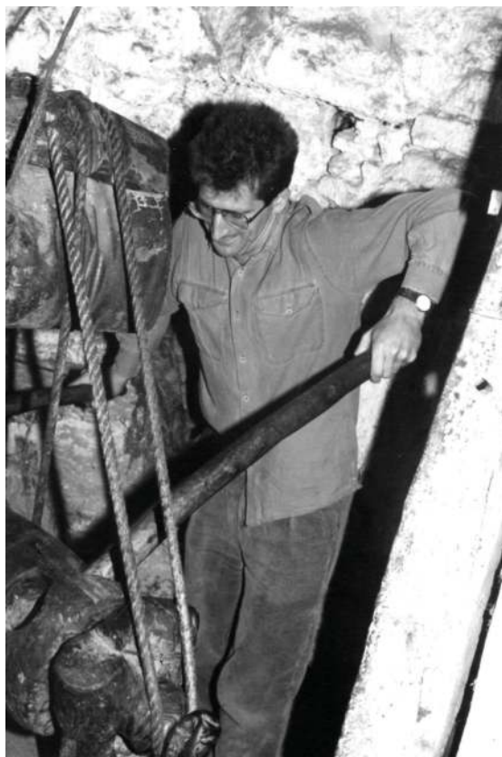
Figure 5.9: A traditional press at Douiret in southern Tunisia in 1987. The way to connect the windlass to the beam press and the use of a handspike to apply pressure (Photo: D. Mattingly).
