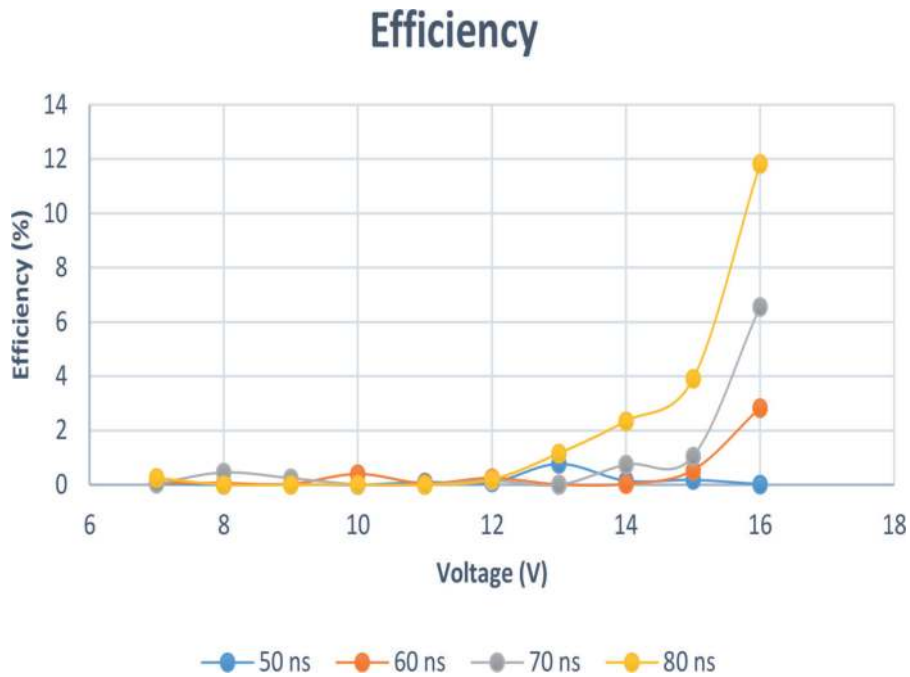
Figure 11. Efficiency of the process as a function of voltage amplitude and pulse on-time.
