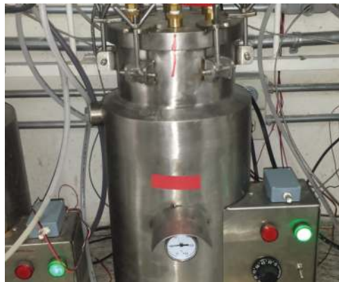
Figure 1. Laboratory-scale anaerobic reactor with pumped circulation.
