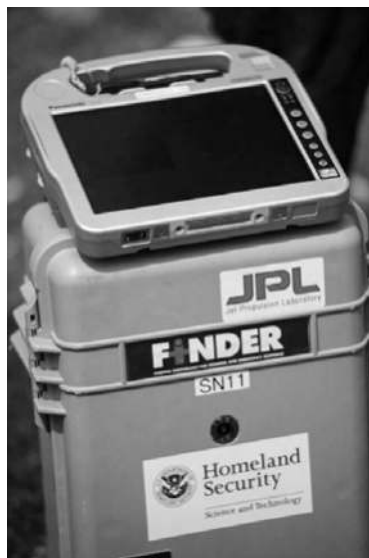
Figure 25.4 Finding Individuals for Disaster and Emergency Response – FINDER radar
