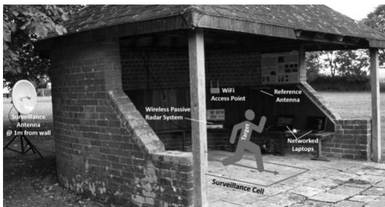
Figure 25.6 Experimental test site for demonstrating the through-wall detection capability of UCL's passive wireless movement detector
