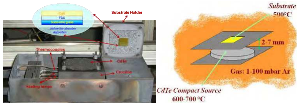
Fig. 2. Picture of the CSS setup used for growing the CdTe films studied (left); Detail of the growth region of the CSS chamber (right).
