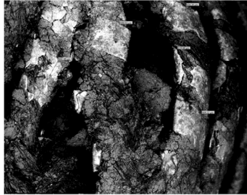
Fig. G.3: Silk core of the thread and metal wrapping revealed
