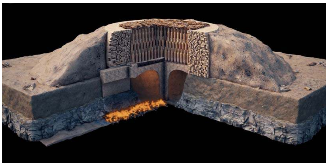
Figure 10. 3D reconstruction of a Mareotid amphora kiln of the Early Empire: developed from the remains of the eastern kiln and parallels, especially Borg el-Arab and Marea-Philoxenite. (Design V. Pichot, modelling and graphics Mohamed Abdel-Aziz, © CEAlex).
