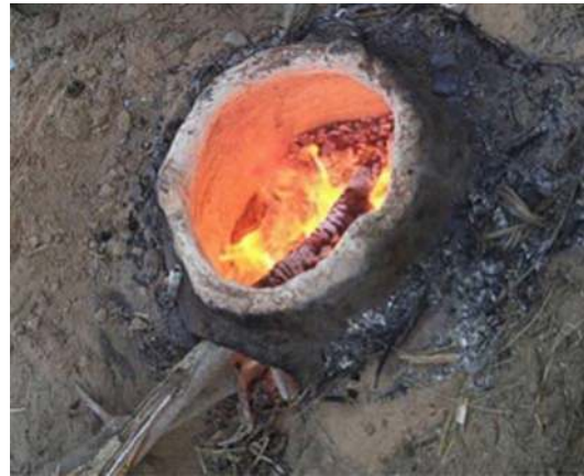
Figure 8. Heating the meefa -oven before its use, photograph by Abu Emeira.
