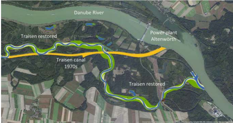
Fig. 15.3 “LIFE+ Project Traisen” in the plan view—Traisen canal from the 1970s (orange) and restored river section (blue) with sediment bars (grey) and both-sided lowered floodplain terrain for river-type-specific riparian vegetation (green) (Source: modified after Technisches Büro Eberstaller GmbH (2010); orthophoto: Copyright © 2014 Esri, DigitalGlobe, Earthstar Geographics, CNES/Airbus DS, GeoEye, USDA FSA, USGS, Getmapping, AeroGrid, IGN, IGP, swisstopo, and the GIS User Community; all rights reserved)
