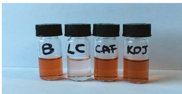
Figure 4. Tyrosinase-catalyzed oxidation mixtures of L-DOPA (1 mM) in the absence (B) or in the presence of 10 \mu\text{M} inhibitor (LC: 2-S-lipoylcaffeic acid; CAF: Caffeic acid; KOJ: Kojic acid).
