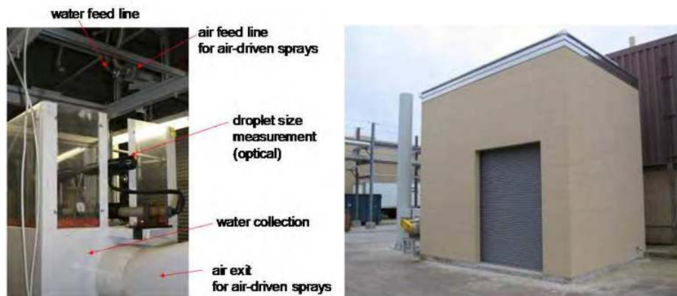
Fig. 1. Interior and exterior view of the nozzle test stand at The Dow Chemical Company, Freeport, Texas, USA.
