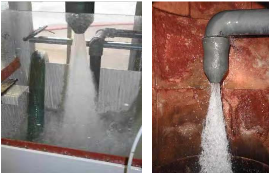
Fig. 2. Left, image of an axially-vaned thermal quench nozzle in operation in the authors' test stand. The aim of this test was to quantify the spray angle and asymmetries of the plant nozzle. Several flow rates and nozzle designs were tested. Right, field test in plant.
