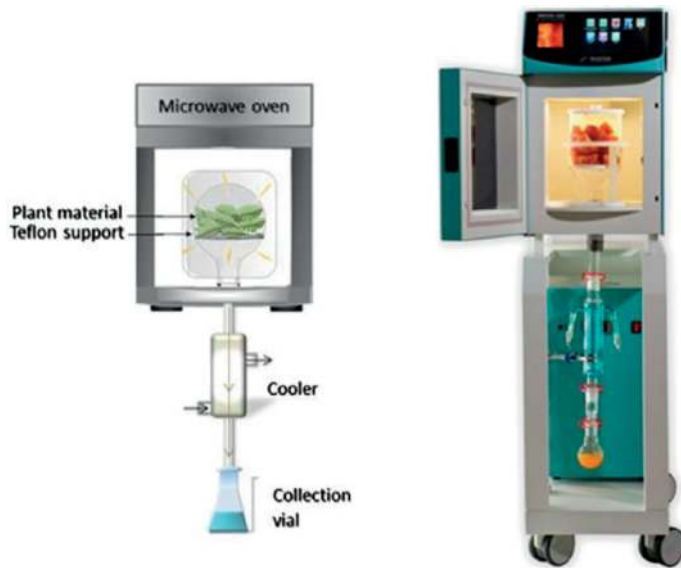
Figure 2. Microwave hydro-diffusion and gravity (MHG) [30].
