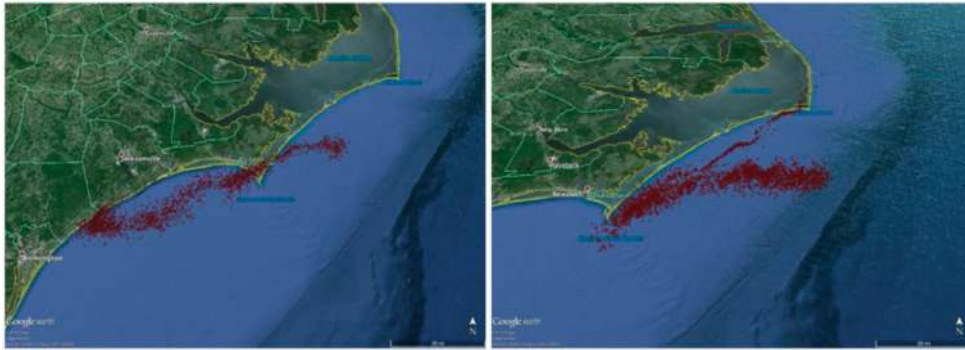
Figure 12. The numerically modeled trajectory of surface oil spills in central Raleigh Bay NC: (a) left panel, shows the surface trajectory of a virtual oil spill driven by an ETC from the middle of the northern bay to the southwest into the lower bay; (b) right panel, shows the surface trajectory of a virtual oil spill offshore and then entrained into a passing GSF. Both wind driven (a) and ocean feature (b) events, project oil being carried to the NC coast. The Red Dots are employed in both panels to depict the trajectories of the oil spilled offshore and carried via surface currents.
