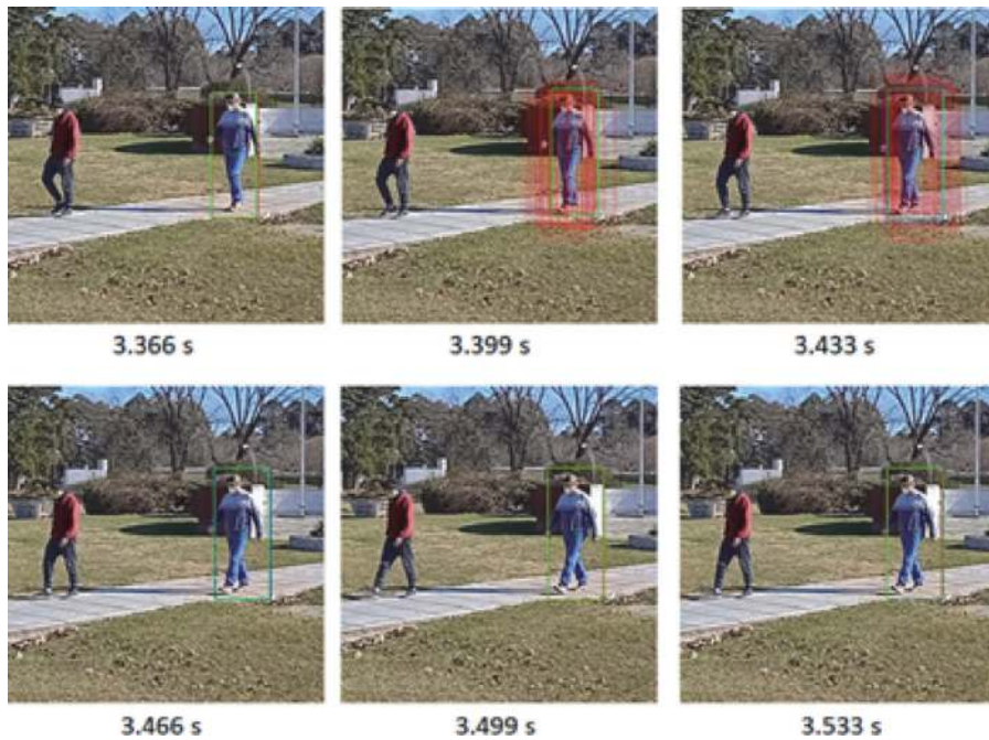
Figure 7. Person tracking, sequence of the particle estimator.
