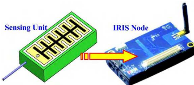
Fig. 23. Self-powered wireless corrosion monitoring sensor
