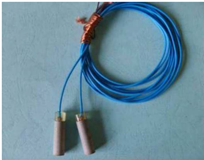
Fig. 19. Solid-state reference electrode
