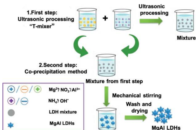
Figure 1. Schematic illustrating the preparation process of MgAl LDHs by hybrid two steps.
