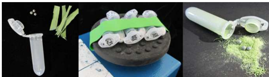
Fig. 14.1 Grinding of plant tissues. Leaf tissue is placed in a 2 ml tube in the presence of metal balls and optional sea sand ( left panel ). Use of desiccated tissue often results in higher-quality DNA compared to fresh tissue. Multiple tubes are then attached to a vortex mixer using tape ( middle panel ). Grinding is complete when a fine powder is produced ( right panel ). The presence of unground tissue with the powder does not affect the quality of extracted DNA
