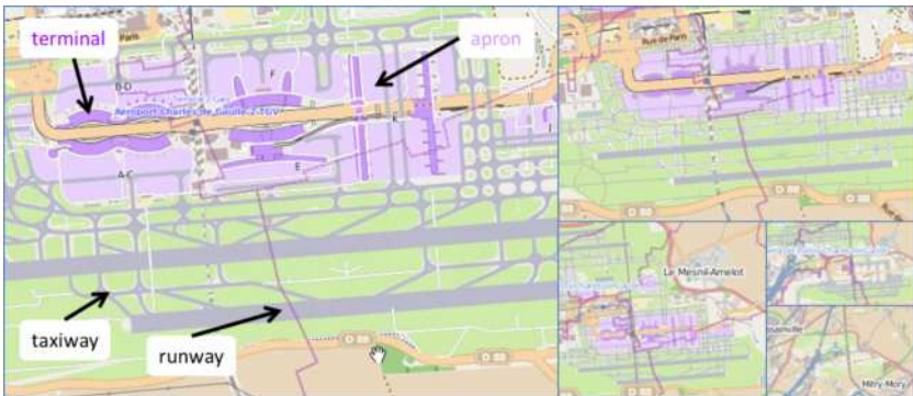
Fig. 5: The complexity of OSM airports composed of terminals, aprons, taxiways and runways, and their representation at several zoom levels. ©Open-StreetMap contributors.
