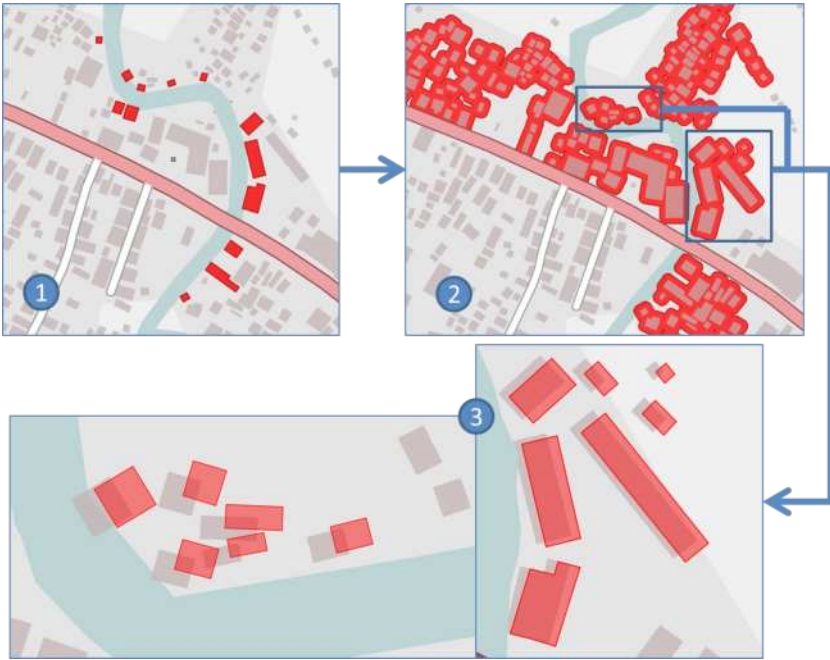
Fig. 16: 1) Detection of LoD inconsistencies (in this case a building intersecting the riverbank); 2) clusters of close buildings are created around the identified inconsistencies; 3) each cluster is harmonised as a whole to remove overlaps without creating new ones. ©OpenStreetMap contributors.
