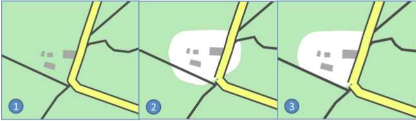
Fig. 15: The roughly digitised forest (1) contains a set overlapping buildings (2), and the newly created clearing is cropped (3) by network sections that often mark the limits of clearings/forests. ©OpenStreetMap contributors.
