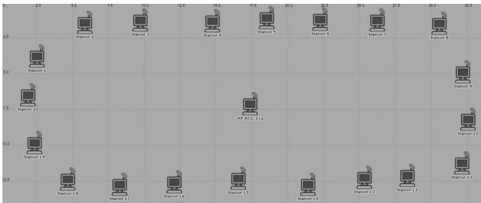
FIGURE 8.4 OPNET representation of WLAN model with 1 AP and 20 wireless stations.
