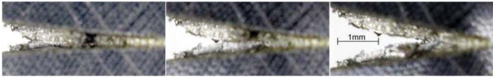
Figure 14. Crack propagation in the chevron-notched zone. The 12GBA tube steel in the UFG state.
