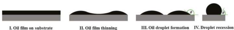
Figure 1. Schematic showing the four stages of oil film dewetting from a uniform thick film (I) to film thinning (II); formation of discrete oil patches (III); and recession of oil patches to form oil droplets at the new equilibrium wetting condition (IV).
