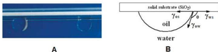
Figure 2. Experimental arrangement employed to measure the effect of cyclodextrins (CDs) on the contact angles. (A) Photograph showing n -dodecane drops in contact with the quartz surface in a cuvette filled with the aqueous phase; (B) Analysis of the drop shape according to the Young equation (Equation (1)), showing the contact-angle (through the water phase) and the interfacial tensions. The solid substrate was a modified quartz surface, the oil drop was n -dodecane and the aqueous phase was a brine solution (0.6 M NaCl) containing dissolved CDs.
