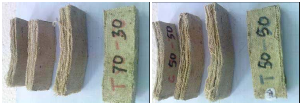
(a) bending specimens biosized 70:30
