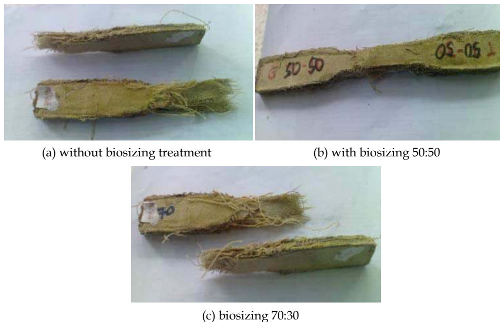
Fig. 6. Failure in biocomposite with different fiber volume fraction
