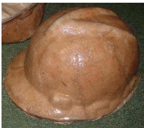
Fig. 11. Preliminary design safety helmet ramie-garut biocomposite
