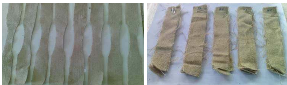
(a) Ramie woven for tensile testing
