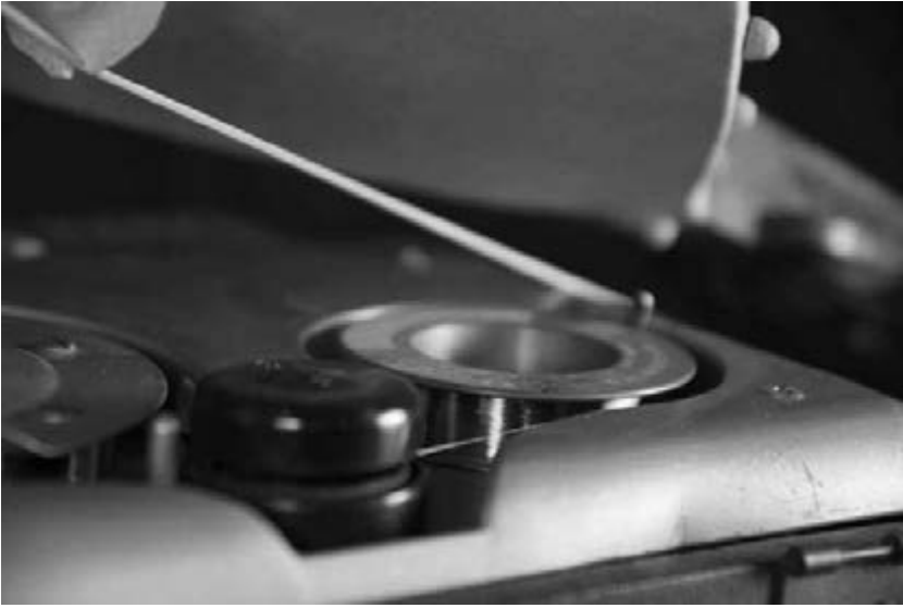
Fig. 1.1: Webster Wire Recorder magnetic spool with the one-string gusle in the background. Photo: Media Archaeological Fundus, Humboldt University, Berlin (Benjamin Renter).
