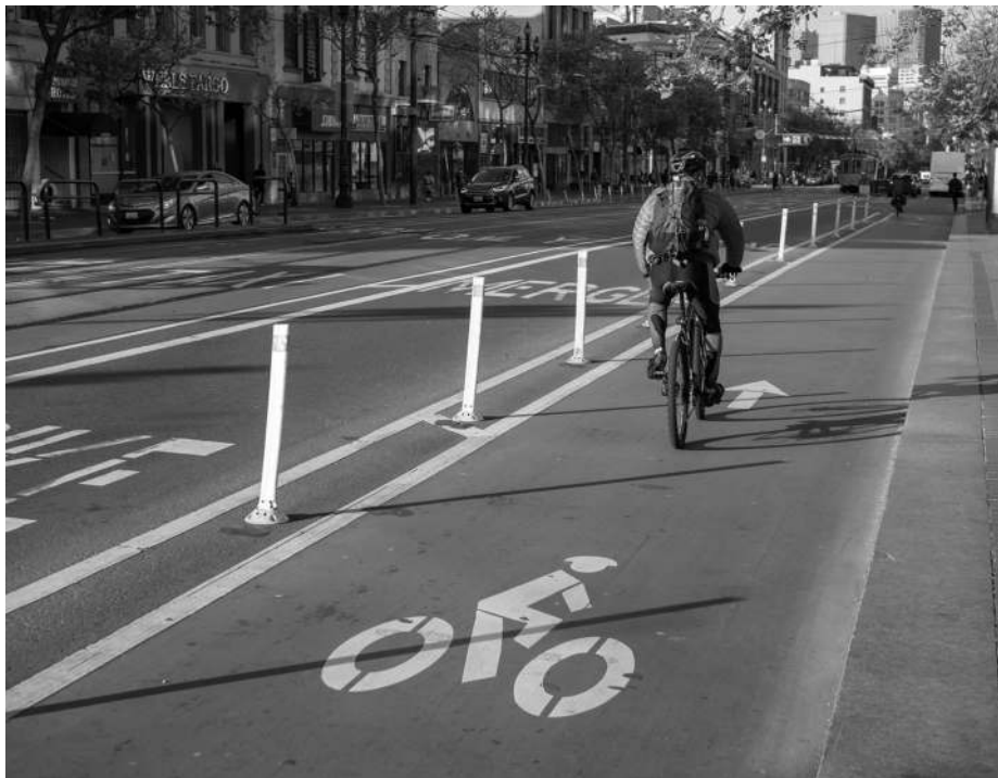
Figure 12.8 Bicycle Lane Along Market Street, San Francisco. To encourage commuting by bicycle, San Francisco has lanes along Market Street, a major city thoroughfare, dedicated to cyclists. Even though the cyclists and cars share a roadway, the bicycle lanes are clearly separated from other lanes, with the green paint and a bicycle icon clearly indicating that these are reserved for cyclists. Plastic barriers or bollards placed along the bike way further help to keep automobile drivers out of the bike lanes, enhancing cyclist safety.
