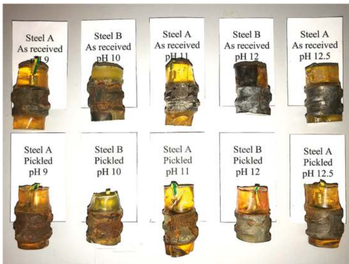
Figure 9. Specimens with as received or pickled surface after the immersion tests at different pH.
