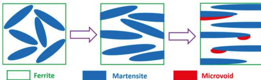
Figure 13. Schematic diagram of microvoid formation in ferrite–martensite dual-phase steel.
