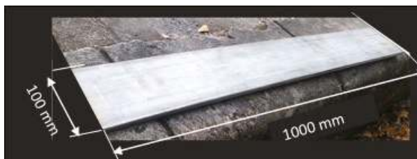
Figure 1. AISI 304 Stainless Steel Strip plate with the dimensions of 1000 mm × 100 mm × 10 mm.
