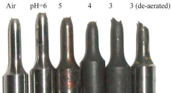
Figure 4. Effect of pH on the fracture morphology of the specimens.
