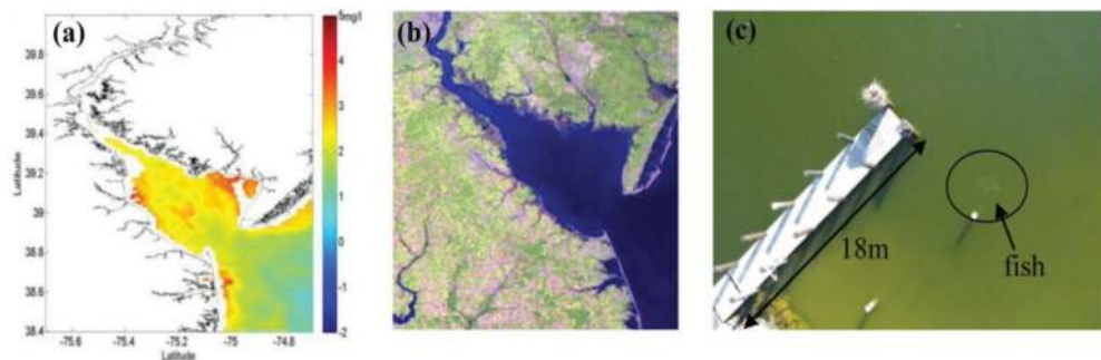
Figure 6. (A) Chlorophyll- a concentration from MODIS at 500-m spatial resolution; (B) combined three bands from ETM+ of Landsat 7 at 30-m spatial resolution; and (C) aerial photo of Helikite at 30-cm spatial resolution in August 31, 2011 (Jo et al. unpublished data) [75].
