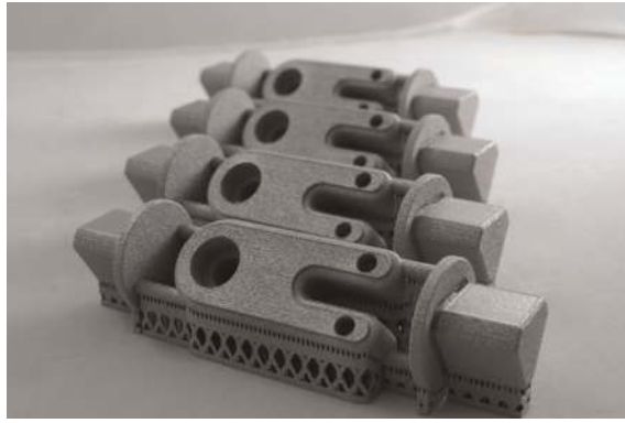
Figure 4. Sample part which could replace multiple components and become part of an assembly after finishing (reproduced from [8]).
