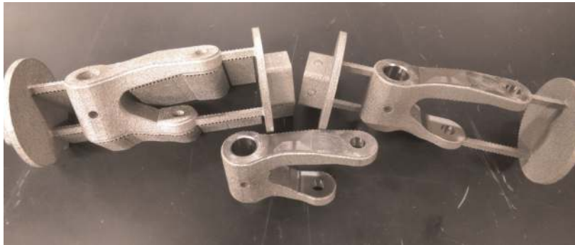
Figure 8. Sacrificial support strategy example part (reproduced with permission from [18]).
