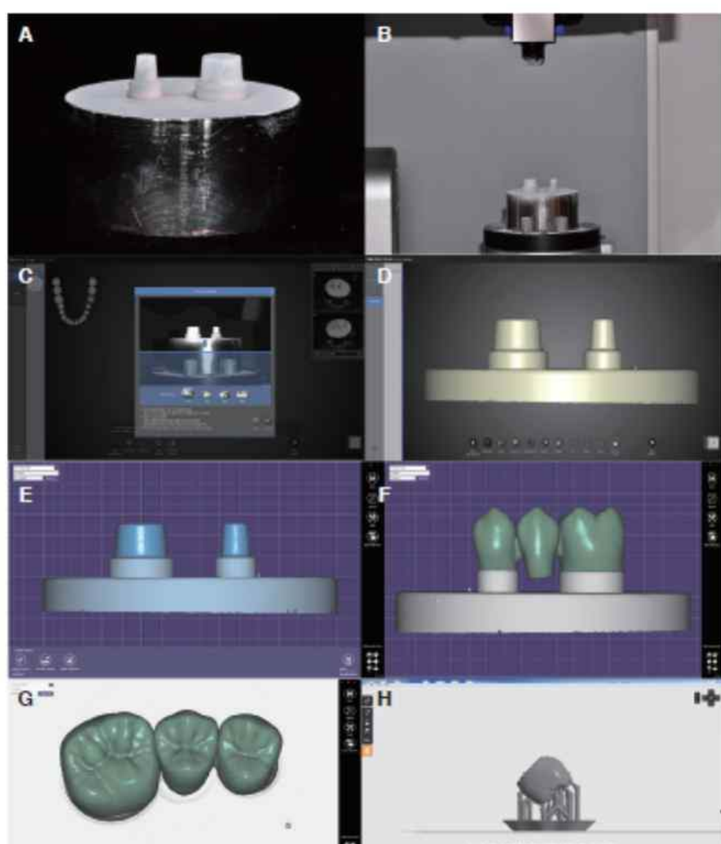
Fig. 2. Procedure of specimen fabrication. (A) Metal jig with IP-scan-spray, (B) Metal jig in the scanner, (C) Scanning area setting, (D) Virtual model of metal jig, (E) Setting cement gap, (F, G) Bridge design, (H) Specimen designed with supporters.
