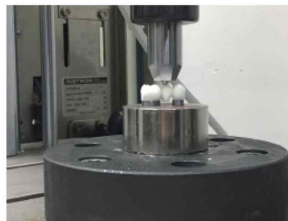
Fig. 3. Flexural strength test of specimen with Universal testing machine.
