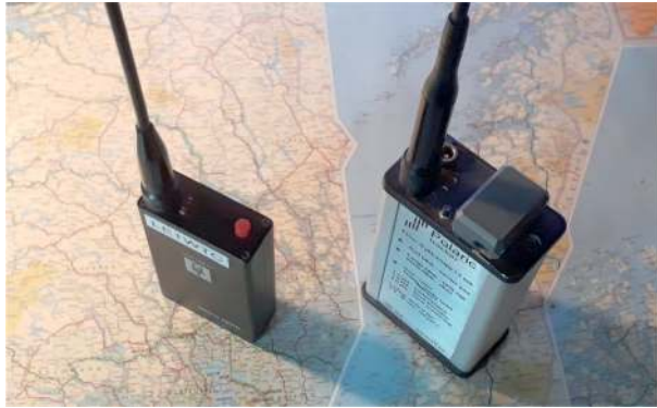
Figure 2. A Polaric Tracker (right side) and a more recent commercial tracker (left side).
