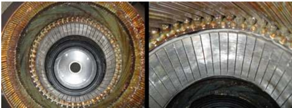
Figure 2. Stator on the side of end-winding connections
