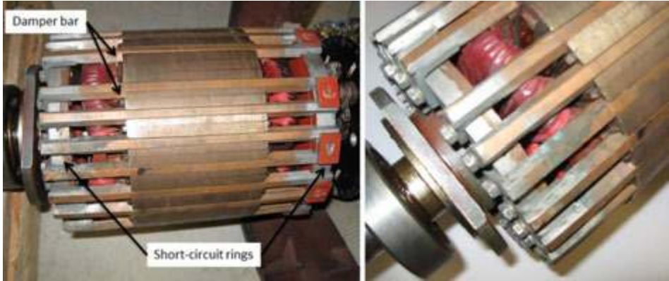
Figure 1. Rotor of the synchronous generator
