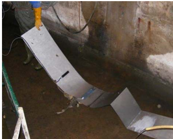
Figure 3.24 An ordinary Doppler sensor (left side, black sensor) and a Doppler profiler (right side, blue-grey sensor) during a comparison campaign. Note the tissues clogging on the connecting wires. Source: Université Gustave Eiffel.
