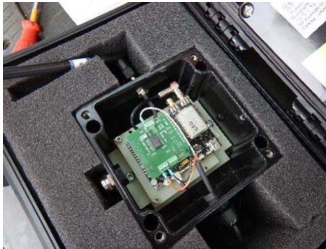
Figure 11.22 Hardware components in LoRaWAN sensor node prototype, embedded in an ATEX compatible chassis. Source: Eawag.
