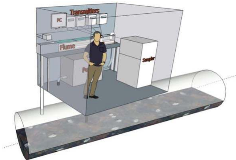
Figure 6.12 3D sketch of the OTHU monitoring station. Source: Nicolas Walcker (INSA Lyon).
