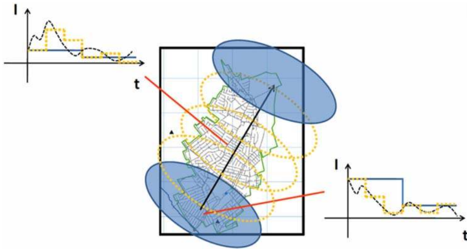
Figure 2.12 Enhancement of radar rainfall estimates for urban hydrology through optical flow temporal interpolation and Bayesian gauge-based adjustment. Source: Wang et al. (2015).
