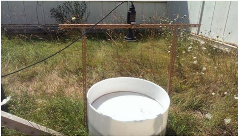
Figure 4.17 Direct measurement of evaporation in a pan by means of a water level radar sensor installed above the pan. Source: courtesy Adama Kone (INSA Lyon).
