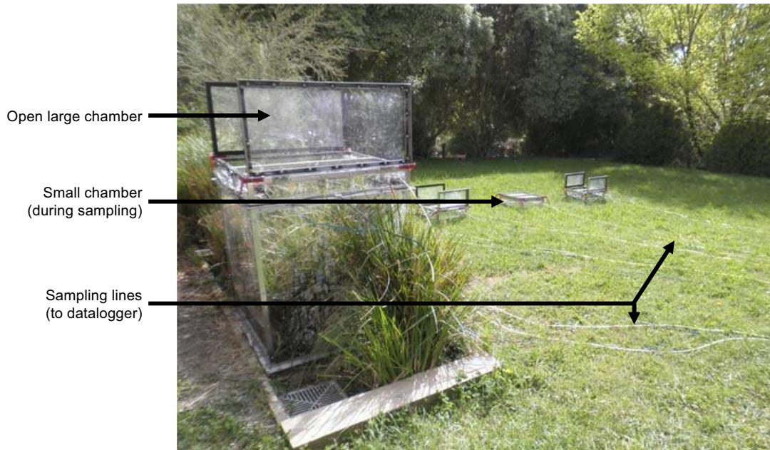
Figure 4.18 Example of application of flux chambers to measure evapotranspiration in a vegetated infiltration system (“rain-garden”) and in surrounding grass. Source: adapted from Hamel et al. (2014) .
