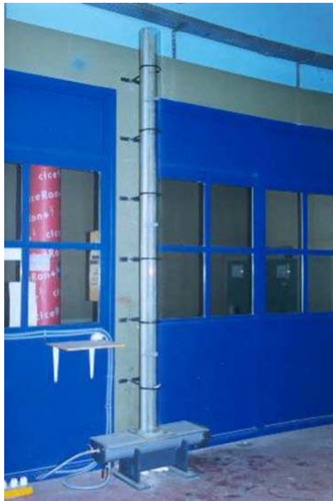
Figure 7.23 Calibration of a water level pressure sensor in a Perspex water column. Source: Jean-Luc Bertrand-Krajewski (INSA Lyon).
