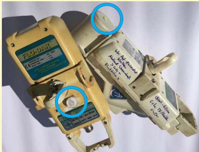
Figure 7.12 Ex situ flow meters (FloDar, Marsh-McBirney/Hach) with a bubble level. Source: Jakob Benisch (TU Dresden).
