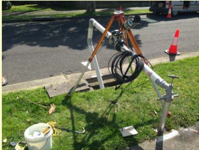
Figure 7.11 Experimental set-up to check discharge measurement devices. Source: Peter Poelsma (University of Melbourne).
