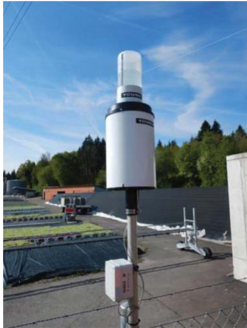
Figure 7.14 R.M. Young tipping bucket rain gauge with calibration bottle. Source: Simon Bloem (Eawag).
