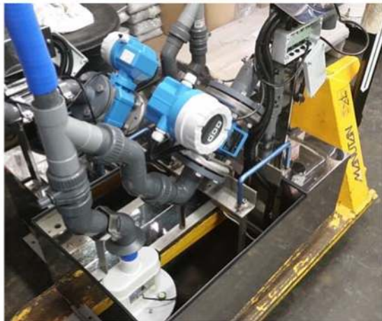
Figure 4.10 (a) installation of a Duo flowmeter to measure the outflow of a green roof; (b) view of a Trio flowmeter. Sources: (a) Rémy Bournique (INSA Lyon & Le Prieuré-Vegetal ID), (b) Le Prieuré-Vegetal ID, Moisy.
