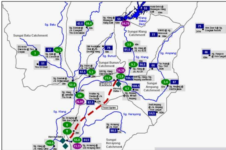
Figure 11.6 A snapshot of the monitoring network within the Klang River catchment, specifically for the operation of SMART. Data for rainfall, water level, and flow velocity are displayed in blue, green, and purple boxes, respectively. The dashed thick red line indicates the SMART Tunnel alignment. Source: Department of Irrigation and Drainage, Malaysia.
