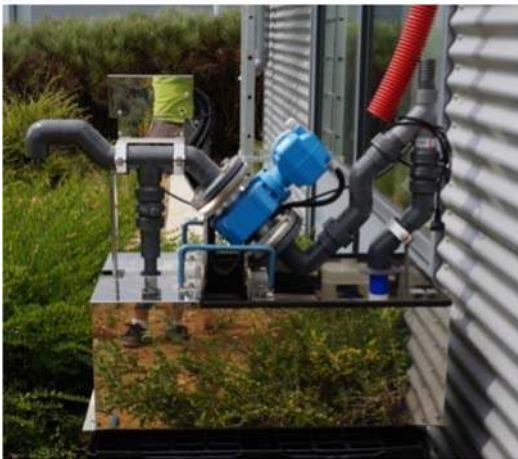
Figure 4.10 (a) installation of a Duo flowmeter to measure the outflow of a green roof; (b) view of a Trio flowmeter. Sources: (a) Rémy Bournique (INSA Lyon & Le Prieuré-Vegetal ID), (b) Le Prieuré-Vegetal ID, Moisy.
