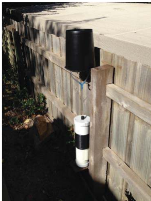
Figure 7.15 Rain gauge with bulk collector used for regular calibration. Source: Peter Poelsma (University of Melbourne).
