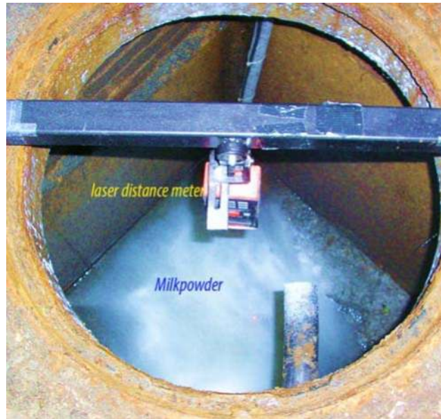
Figure 7.18 Measuring water level with a laser meter and milk powder. Source: courtesy of Francois Clemens-Meyer (Deltares/TU Delft/NTNU).
