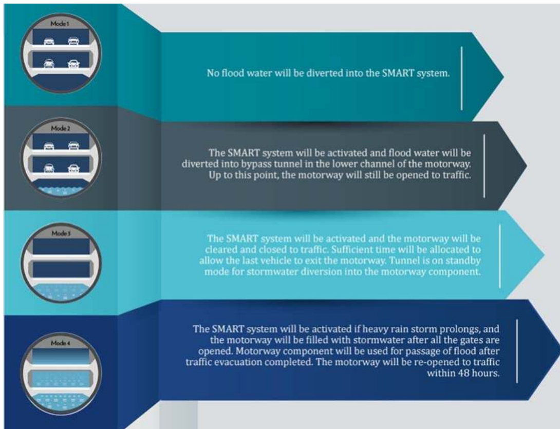
Figure 11.3 Four modes of SMART operation. Source: Department of Irrigation and Drainage, Malaysia.
