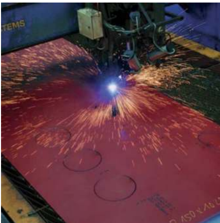
FIG. 71 The reduction to some standard steel sheets and profiles allow in combination with computer controlled plasma-cutters a high customisation. [source: www.meyerwerft.de]
