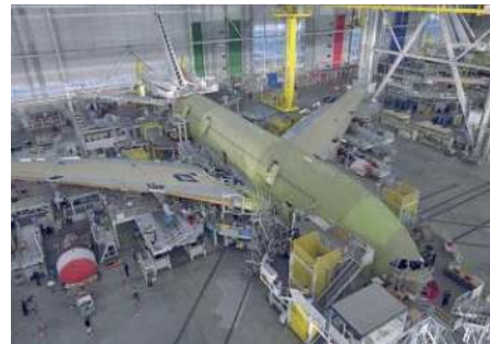
FIG. 76 Final assembly of the Airbus A 380 takes place in Toulouse. [source: www.airbus.com]
