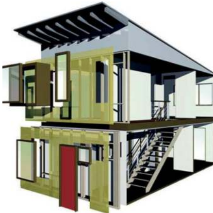
FIG. 113 Optima Homes represent a timber-frame based customizable panel building system. [source: www.optimahomes.co.uk ]
