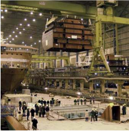
FIG. 69 A 6-storey high prefabricated part of the ship is craned to the main hull. [source: www.meyerwerft.de]
