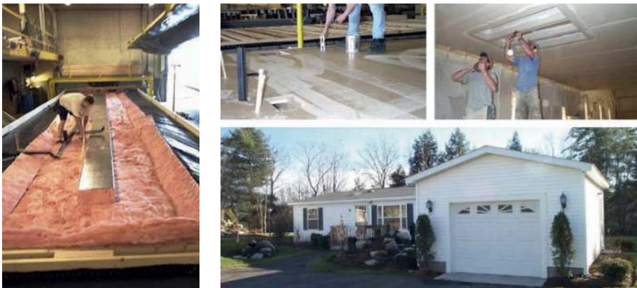
FIG. 49 Example images of manufactured home production, which still involves a lot of ergonomically unfavourable manual work [source: www.skylinehomes.com ]
