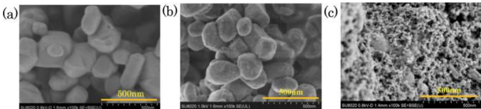
Figure 16. FE-SEM images of titanium oxide particles (a) as-received, (b) after WJ processing, (c) after MFC processing ( \times 100,000 ).
