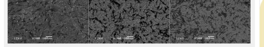
s-Ti r-Ti r-Dopa While both r-Ti and r-Dopa showed microporous titanium consisting of steep-sided pores or sharp triangular peaks, there was intact titanium surface in s-Ti. In terms of cell morphological outcomes, there was no distinctive difference among the groups. Tense HGF proliferation was present in the surface of r-Dopa.
