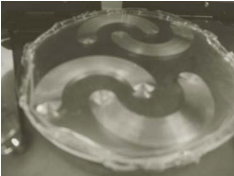
FIGURE 10.8 Example of a PDMS mold produced from the silicon master.
