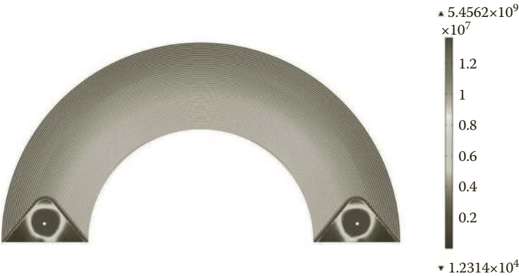
FIGURE 10.4 (See color insert.) Meniscus design with channels 100 \mu\text{m} wide separated by PDMS barriers that are 100 \mu\text{m} thick. Gradient of the inner product of the electric field modeled at 5 V and 1 Hz.
