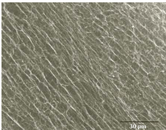
FIGURE 10.2 Aligned bacterial cellulose nanofibers.
